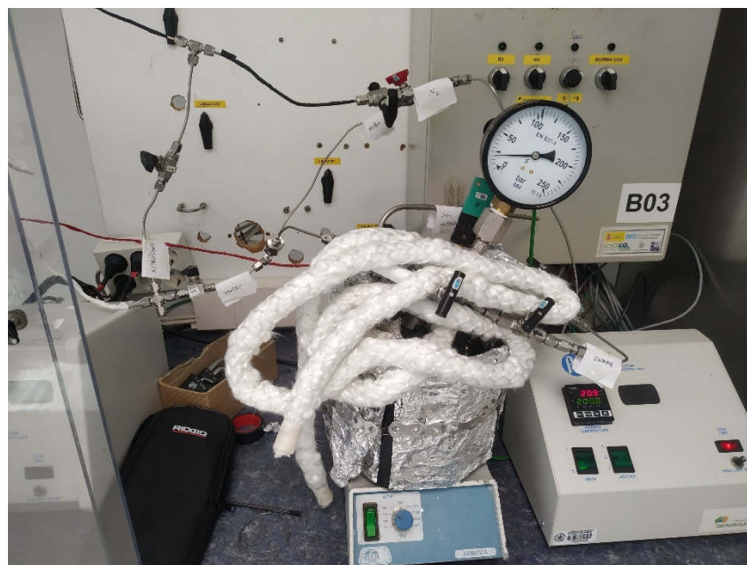
Fig. 2.: Image of the 25 mL reactor
