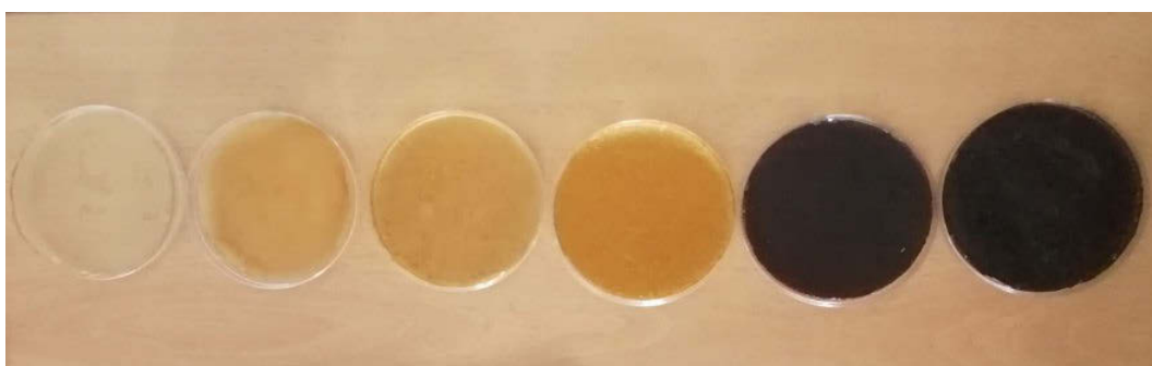
Figure 1. Soy film and bio-based films reinforced with 5% fibre obtained under different hydrolysis conditions (C1-C5).
