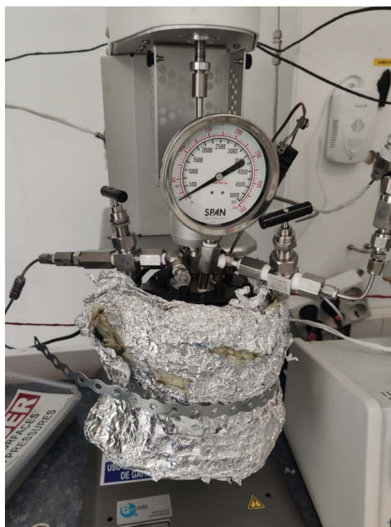
Fig. 2.: Image of the 50 mL reactor
