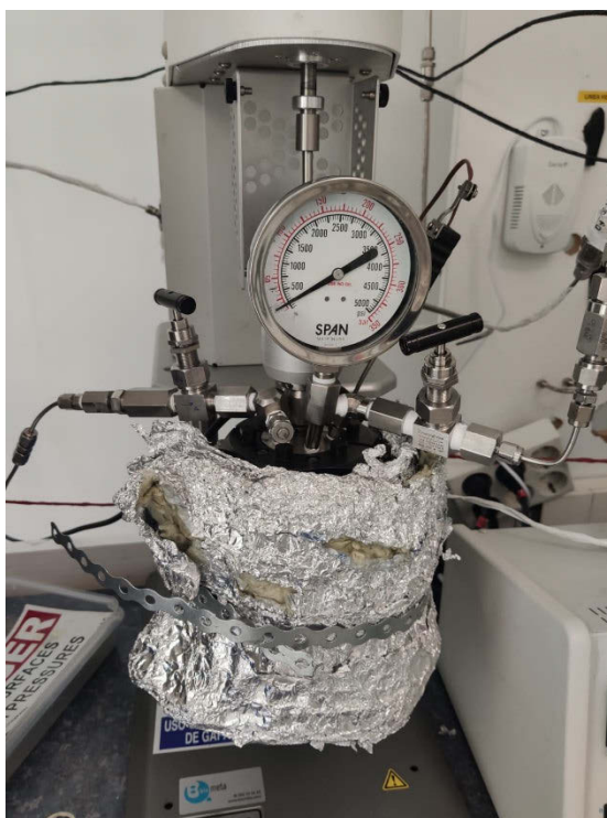
Fig. 2.: Image of the 50 mL reactor
