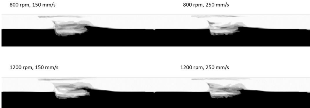
Fig. 8 Contour plot of a transverse section post welding; the grey scale shows the mixing of the top and bottom plates; for the conventional threaded tool
