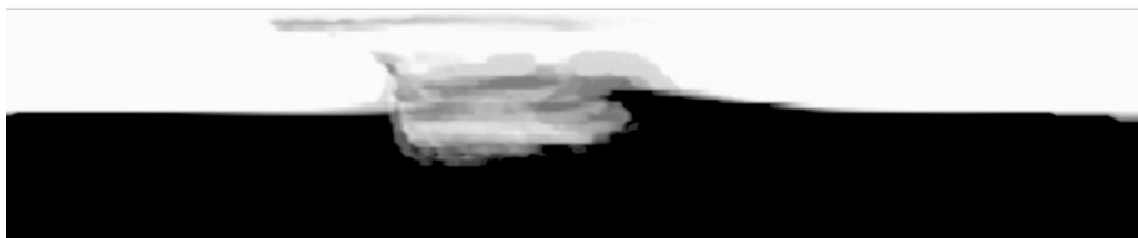
Fig. 6 Contour plot of a transverse section post welding; colours show the mixing of the top and bottom plates; for the conventional threaded tool at 1200rpm and 250mm/min
