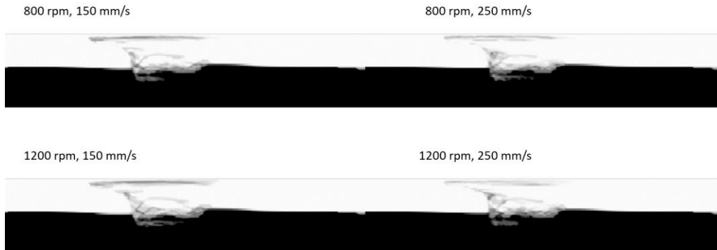
Fig. 10 Contour plot of a transverse section post welding; grey scale shows the mixing of the top and bottom plates; for the mixed threaded tool
