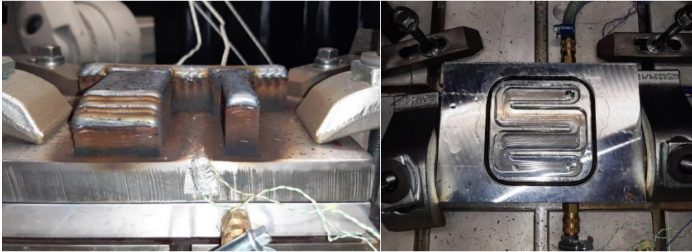
Fig. 2 (a) Clamped welded part (b) Cooling plate
