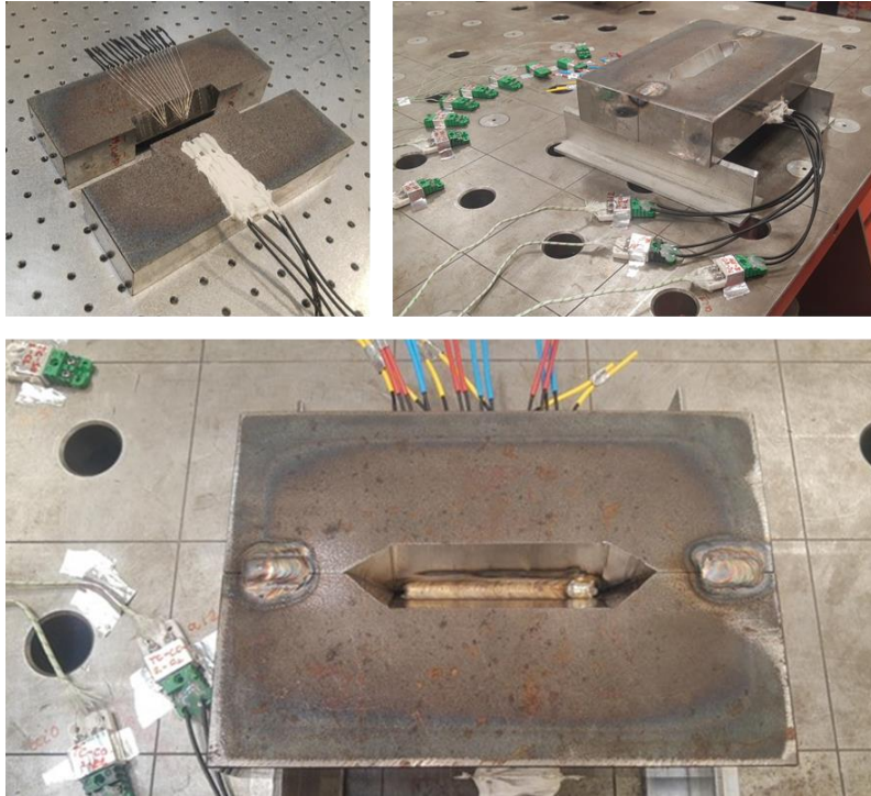
Fig. 10 The thermocouple-instrumented mock-up before assembly and after the welding run completion
