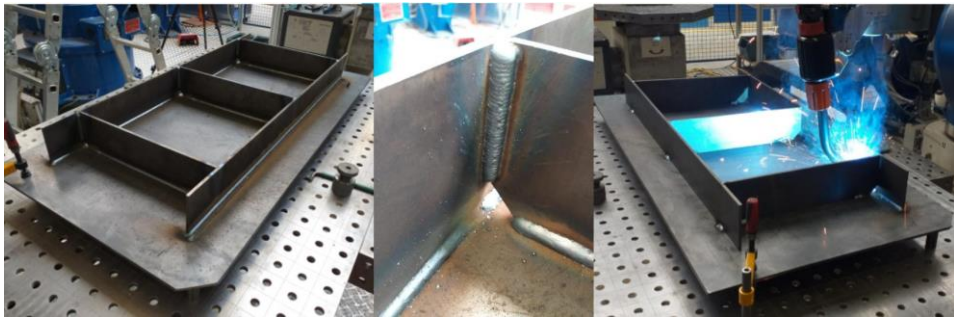
Fig. 1 Test specimen - TIME stiffened plate
