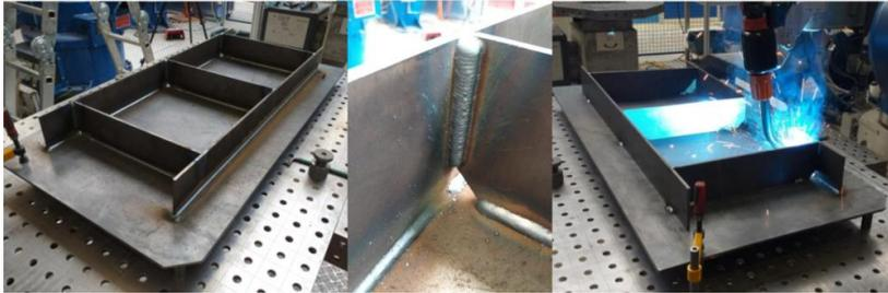
**Fig. 1** Test specimen - TIME stiffened plate
