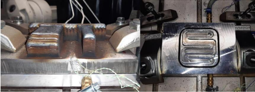
**Fig. 2** (a) Clamped welded part (b) Cooling plate
