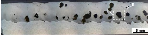
**Fig. 4** Longitudinal section of LBWed joints of 5754 aluminum alloy
