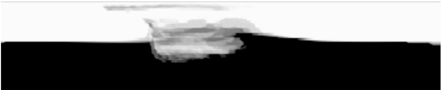
**Fig. 6** Contour plot of a transverse section post welding; colours show the mixing of the top and bottom plates; for the conventional threaded tool at 1200rpm and 250mm/min
