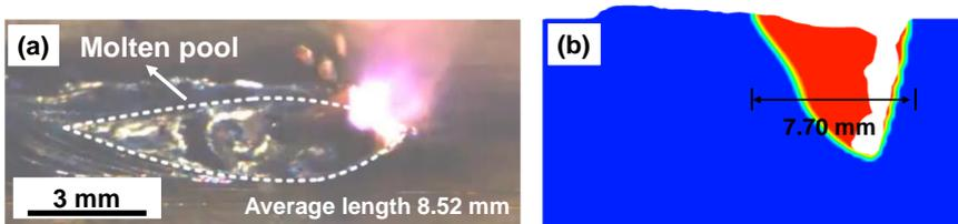
**Fig. 5** Comparison between experimental and calculated molten pool length without magnetic fields: (a) experiment results; (b) calculated results (the red region in the simulation result represents the calculated weld region)
