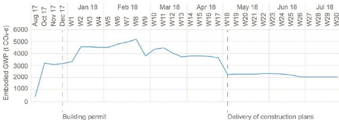
Figure 19: Evolution of total results for embodied GWP in t CO<sub>2</sub>-e throughout the design process. Source: (Hollberg, Genova, et al., 2020).
