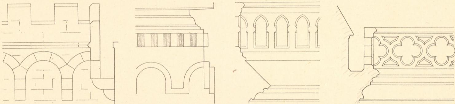
•FIG. 18• GOT KONSOLEN GESIMSE • FIG. 19 • GURTGESIMSE ROM • SOCKELGESIMSE GOT • FIG. 20 • GURTGESIMSE GOT • FIG. 21 • GOT KONSOLEN GESIMSE •
