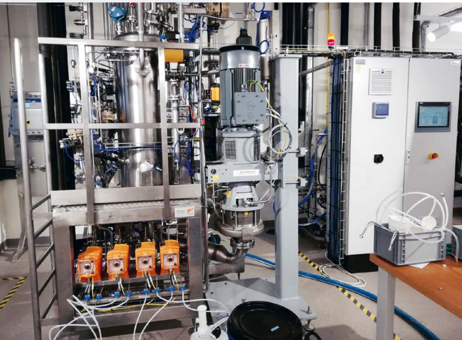
Figure 3: Pilot gas bioreactor at 300 L volume capacity.
