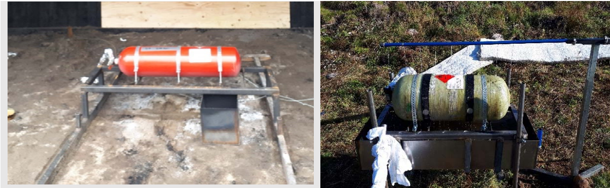
Figure 1. Left: small fire pan (i.e. local fire exposure) below CNG steel tank. Right: application of water onto CNG composite tank with widespread fire pan below the tank. (Photo: RISE)
