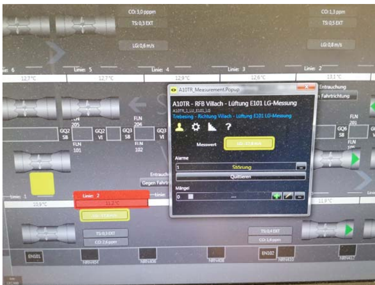
Fig. 2: Example: LG measuring device malfunction during fire simulation
