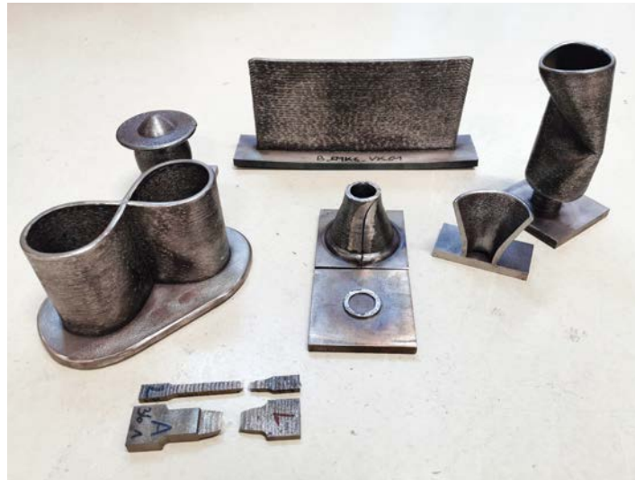
Figure 1: 3D printed metallic materials, from the FFG project entitled "3D Welding: Additive Fabrication of Structural Steel Elements", which funds the PhD research from Christoph Holzinger.
