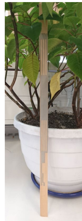
b) Printed antenna on wood carrier
