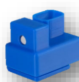
Figure 3: H 2 ambient gas sensor - laboratory sample, NIP2-project H2D4EV
