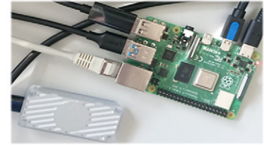
Fig. 3: HW setup used for experiments: Raspberry Pi 4 and Google Coral Edge TPU
