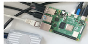
Fig. 3: HW setup used for experiments: Raspberry Pi 4 and Google Coral Edge TPU
