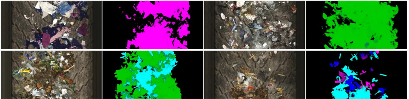
Fig. 1. Mono-material stream samples and binary segmentation belt/waste (top row) and synthetic ground-truth data with mixed stream (bottom row). All images: plastics (green), wood (turquoise), textiles (purple), paper (blue).
