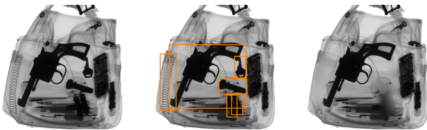
Fig. 1. From left to right: original scan, detected benign and threat objects, and distractor removal applied with Regionfill .
