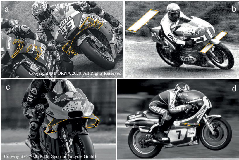
Figure 2.6: Examples of Grand Prix racing motorcycle downforce devices. a) Honda RC213V and Ducati GP19 from 2019 [14], b) Rodger Freeth and his concept 'Aerofoil Vitko TZ750A' from 1977 [61], c) KTM RC16 from 2019 [35] (aerodynamic design by the author) and d) Barry Sheenes' Suzuki RG500 from 1979 [58].
