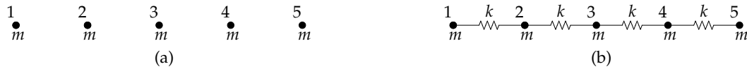
Fig. A.1.: (a) One dimensional chain of five atoms and (b) its approximation as a spring-mass system.
