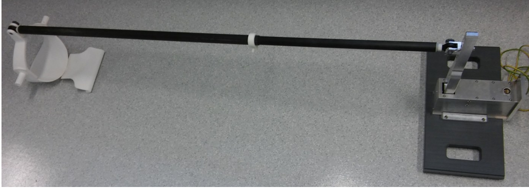
Figure 2.3: The piezoceramic actuator coupled to a head rocker via a carbon fiber rod.
