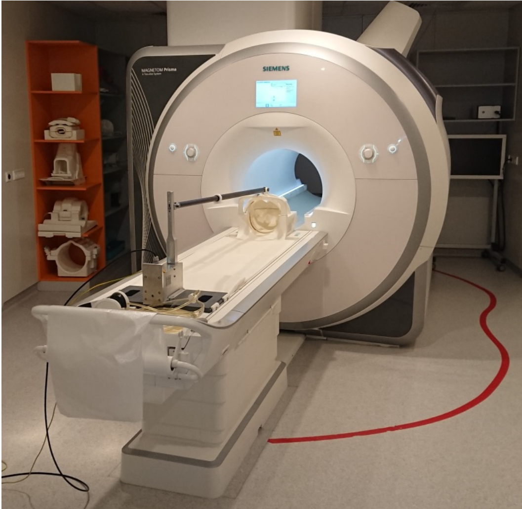
Figure 2.5: The excitation device mounted on the patient table of the MR scanner.
