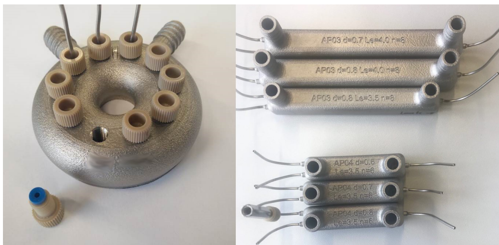
Supporting Information Figure S4.2: Pictures of the SLM printed CSTR cascade with inserted HPLC flat bottom connectors (left) and various parameter reactors AP03 and AP04 with different length scales and internal diameters (right).
