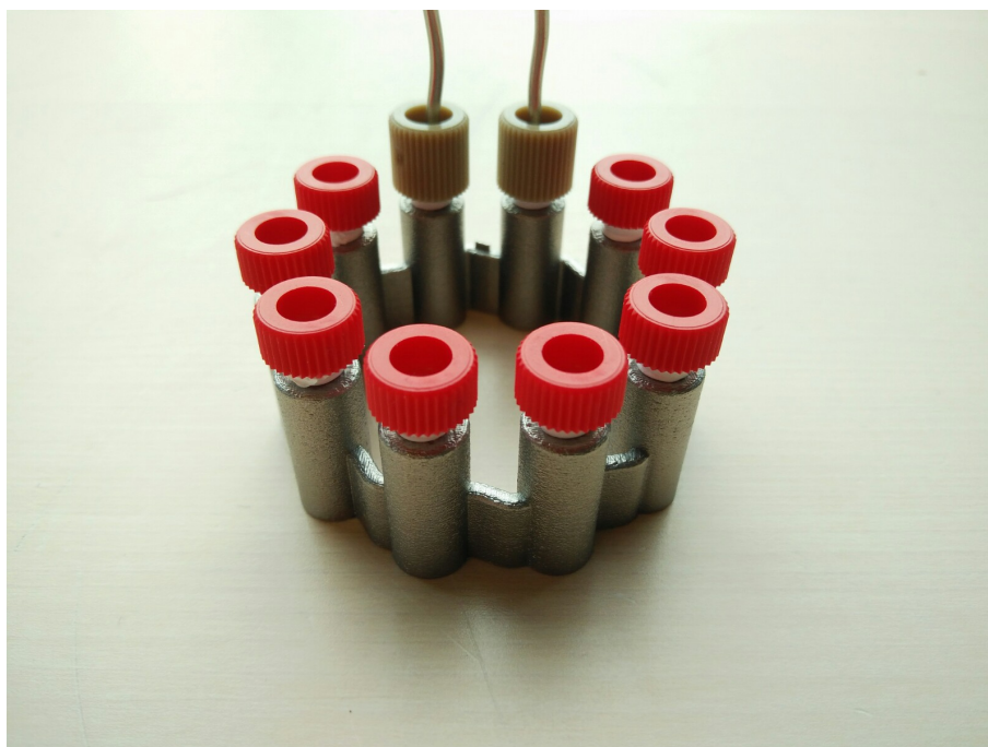
Figure 2.6: 3D printed CSTR cascade (AP01) closed with standard HPLC fittings. The 3D printed 10-32 UNF thread had to be refined after the printing.
