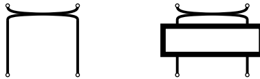
Figure I.B.15. Graphical representation of a swap gate (left) and a combination of a swap gate and a general operator that acts on two neighboring sites (right).
