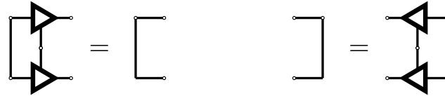
Figure I.B.9. Graphical representation of a left-normalized tensor and a right-normalized tensor. Triangles pointing to the right are left-normalized tensors (because they collapse to the right when contracting), while triangles pointing to the left are right-normalized tensors.
