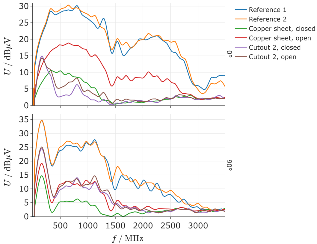
Figure 3.13: Envelope of the TEM cell spectra of the TOF sensor shielded with copper tape in the configurations with the copper sheet and cutout 2.
