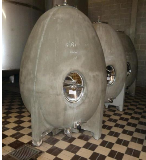
Figure 41: Egg shaped concrete tanks (Grainger and Tattersall 2016)
