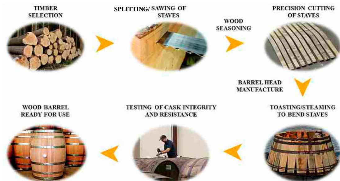
Figure 36: Barrel manufacturing process (Carpena et al. 2020, p. 6)
