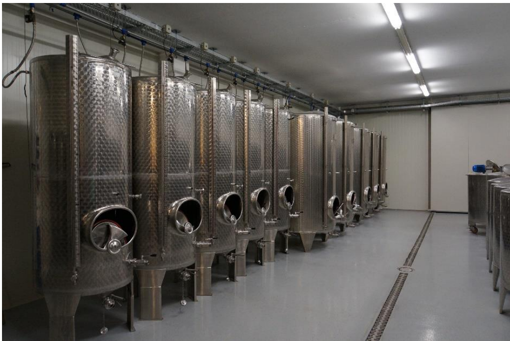
Figure 38: Stainless steel tanks for fermentation and storage of wine in Styrian winery
