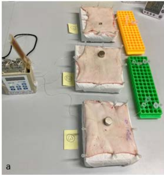
Figure 29: Experimental setup of the ex vivo experiment using porcine skin flaps. (a) Position 1-3) with magnet type 2 applied on position 1 and magnet type 1 on positions 2 and 3; (b) Position 3 with magnet type 1 applied. The tube was implanted into a depth of 3.46 mm
