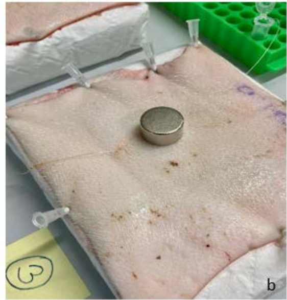
Figure 29: Experimental setup of the ex vivo experiment using porcine skin flaps. (a) Position 1-3) with magnet type 2 applied on position 1 and magnet type 1 on positions 2 and 3; (b) Position 3 with magnet type 1 applied. The tube was implanted into a depth of 3.46 mm
