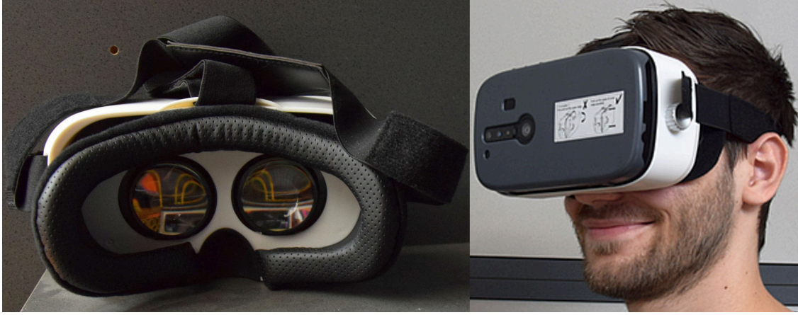
Figure 7.4: Untethered smartphone-based headset prototype based on the Qualcomm Snapdragon™ 835 Mobile Platform, with a resolution of 2560 \times 1440 , displaying a stereo view of the Robot Lab scene.
