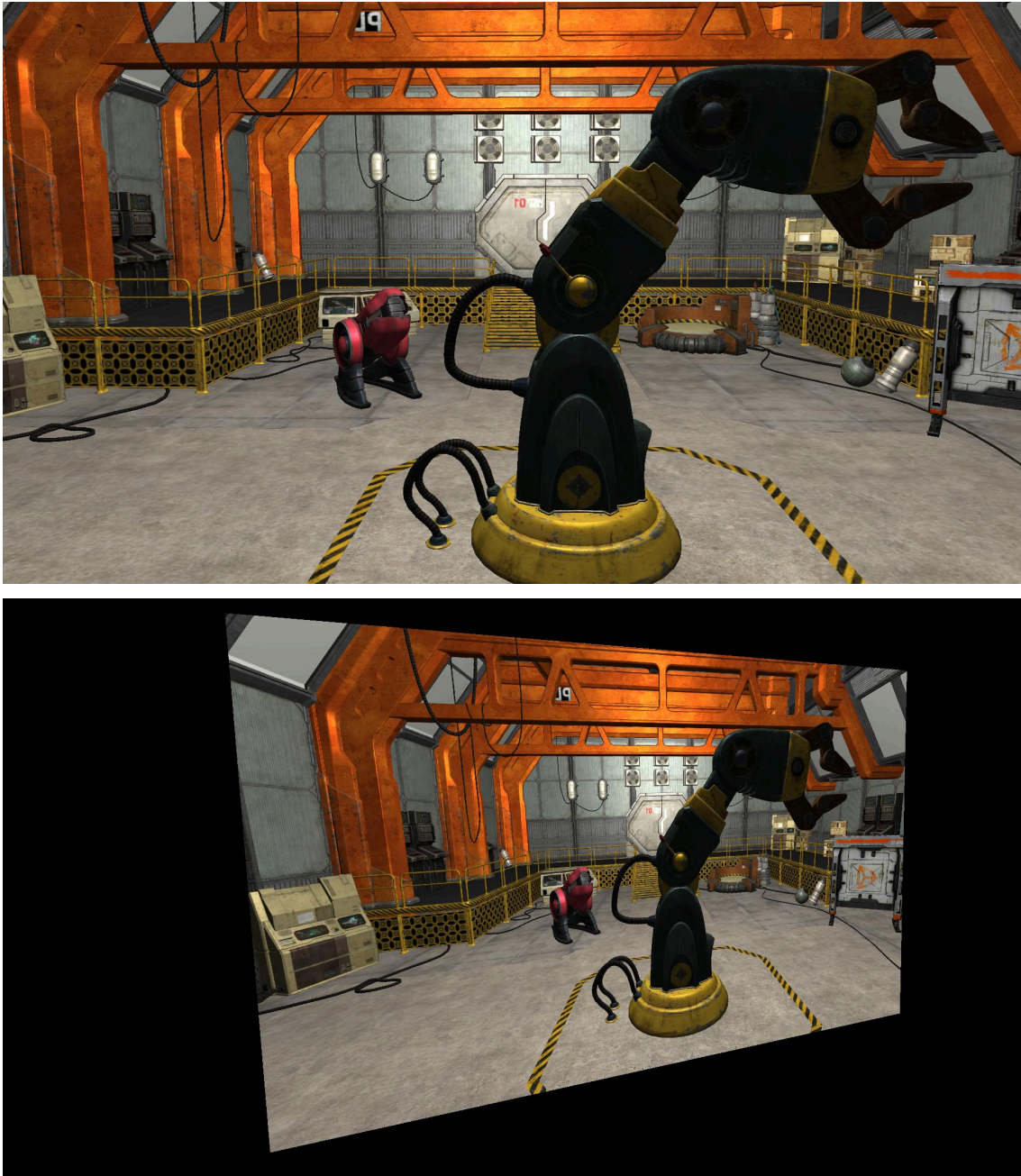
Figure 2.1: Asynchronous time warping [107] simple warps the image plane in accordance with the camera movement. A slight sideward translation (top) moves the whole image at the same rate, without considering the distance of the objects within the scene. Further translation of the camera (bottom) reveals the flat image plane that ATW is using.
