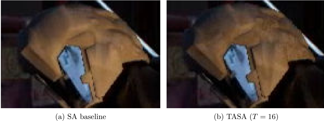
Figure 6.5: An example of an artifact of the TASA proof of concept running in VR: (a) Ground truth shading of a light fading to black after having a constant intensity for several seconds. (b) The lighting on the helmet is not updating uniformly due to TASA wrongly predicting the shading time, resulting in artifacts at geometric borders.
