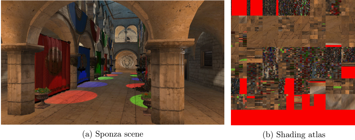
Figure 1.3: The sponza scene (a) is rendered with the shading atlas (b) that stores the shading of the visible geometry.
