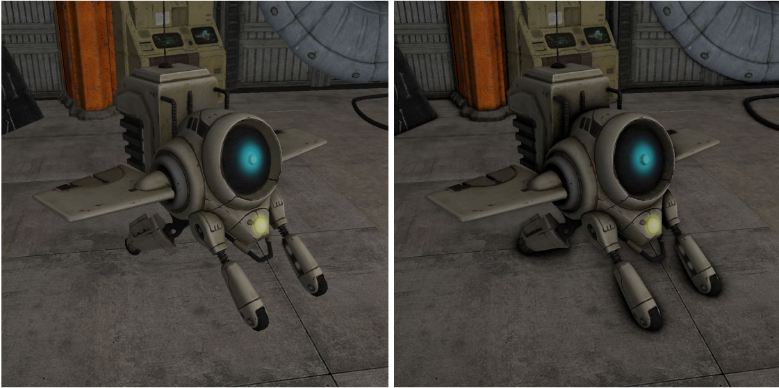
Figure 7.12: To demonstrate how postprocessing effects can be integrated into SAS, we added screen-space ambient occlusion (SSAO) to the shading stage. The screenshots show Phong shaded images without (left) and with (right) SSAO.
