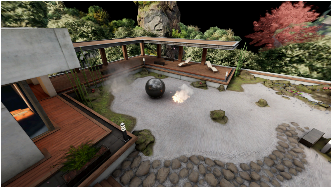
Figure 7.11: The shading atlas streaming server renders particle effects of Epis’s “Epic Zen Garden” scene as transparent billboard which are streamed to the client. The client simply renders the transparent billboards like any other transparent geometry. Image courtesy of Wolfgang Tatzgern.
