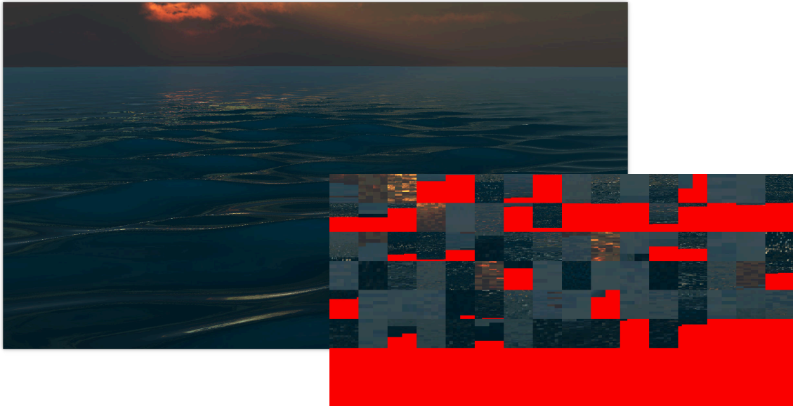
Figure 7.13: The “water scene” contains an ocean surface with animated waves. The waves are animated in the vertex shader depending on the current time. Our shading atlas streaming system supports this dynamic geometry by transmitting the updated vertex positions to the client.
