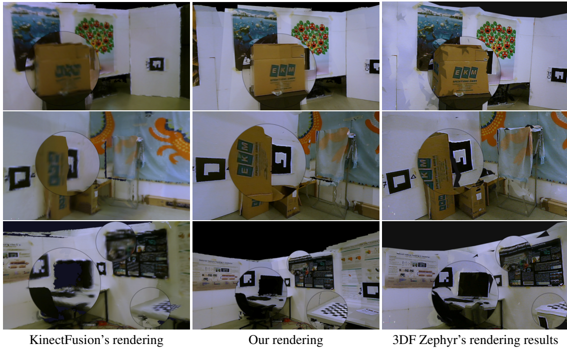
Figure 3.16: Comparison of our method to per-vertex colored KinectFusion model and to an offline-reconstruction rendering using a leading commercial photogrammetry software (3DF Zephyr).
