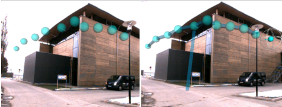
Figure 2.7: Zollmann et al. visualize drone's altitude over the terrain and distance to the user in 3D.
