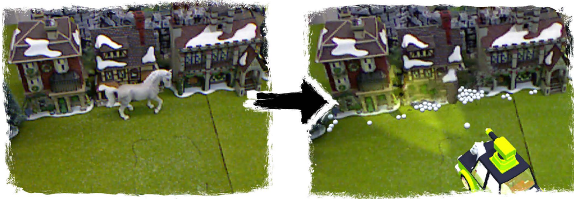
Figure 4.1: 3D diminished reality followed by augmented reality rendering. Our system, InpaintFusion , is able to remove objects and inpaint color and depth information. While previous attempts for real-time inpainting are limited to color channel inpainting only, InpaintFusion supports arbitrary depth channel inpainting as well. As it provides depth information, 3D augmented reality rendering in the inpainted environment becomes possible. This example shows a real white horse in front of a set of houses (left). We inpaint the color and depth values of the horse (right). This enables us to add a virtual car with head lights to illuminate the inpainted regions, together with white balls which can interact with the inpainted region by bouncing of the walls.
