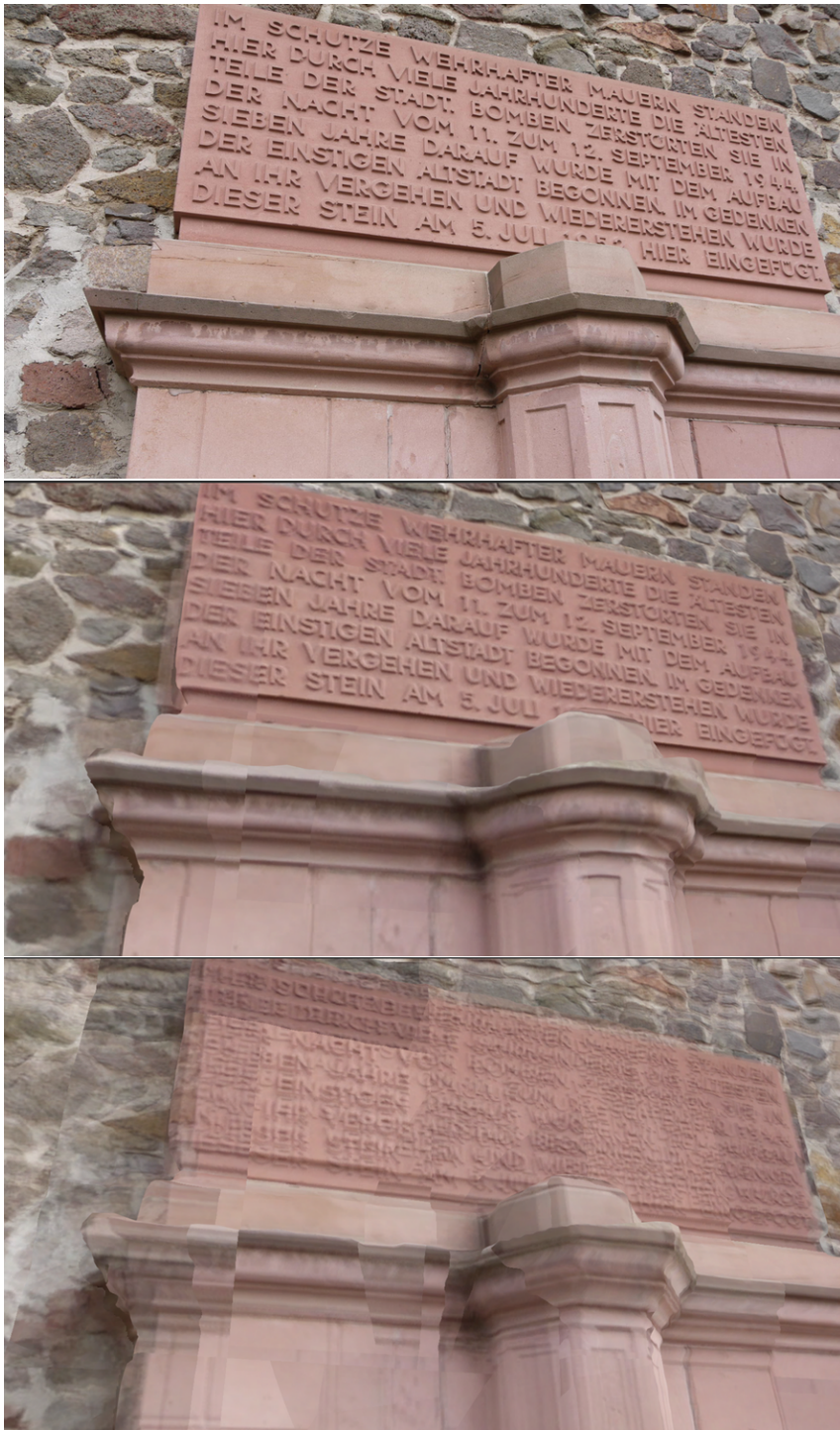
Figure 3.7: Quality comparison of “city wall” scene, from top to bottom: ground truth, lumigraph rendering with view processing (pose and exposure refinement), lumigraph rendering without view processing. In the latter case, blurriness and exposure differences reduce image quality.
