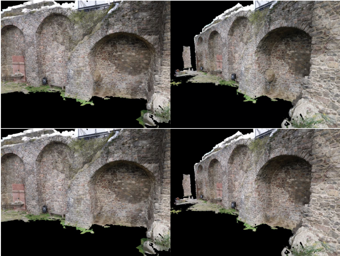
Figure 4.17: Removing a historical cannon ball from a city wall, rendered using our IBMR pipeline.
