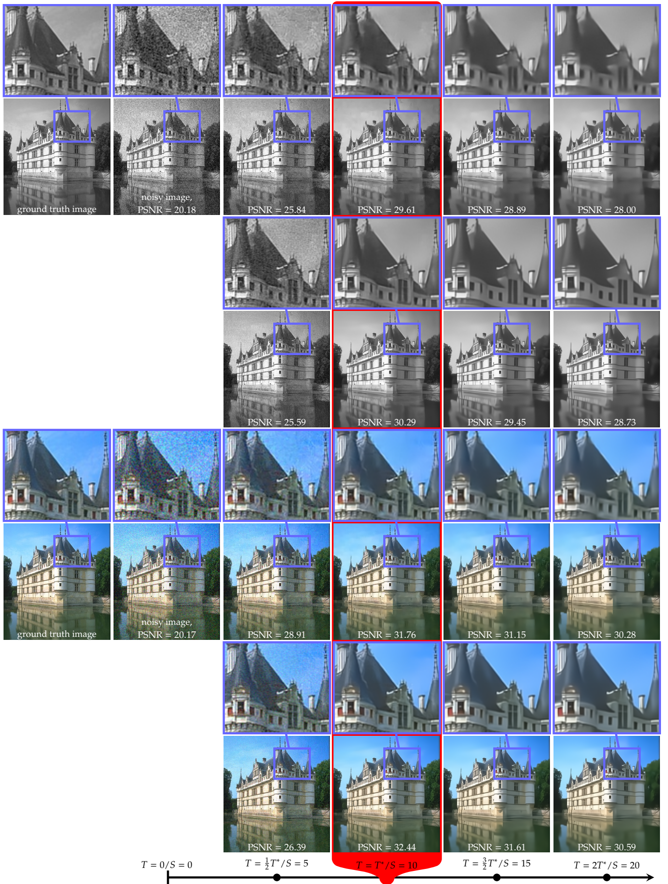
Figure 6.5: From left to right: Ground truth, noisy input with noise level \sigma = 25 and resulting output of the learned regularizers for (S, T) \in \{(5, \frac{1}{2}T^*), (10, T^*), (15, \frac{3}{2}T^*), (20, 2T^*)\} . First row: FoE 48 for gray-scale Gaussian denoising. Second row: TDV 3 for gray-scale Gaussian denoising. Third row: FoE 48 for color Gaussian denoising. Fourth row: TDV 3 for color Gaussian denoising. Note that the best images are framed in red and are obtained at the learned optimal stopping time T^* .
