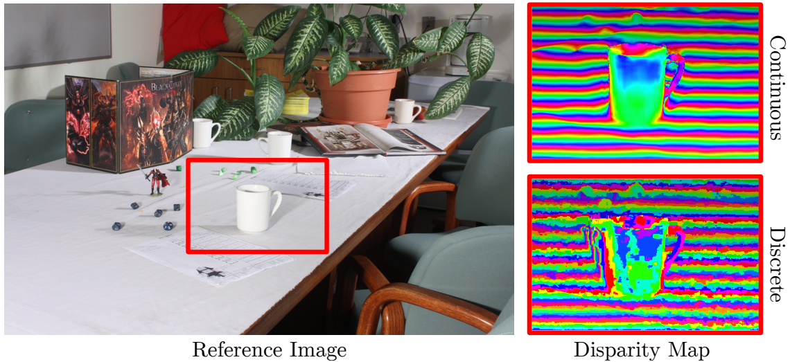
Figure 2.27: Comparison between discrete and continuous stereo. The disparity maps are shown using a high-frequency visualization to highlight the disparity changes. Images from [85] and [84].
