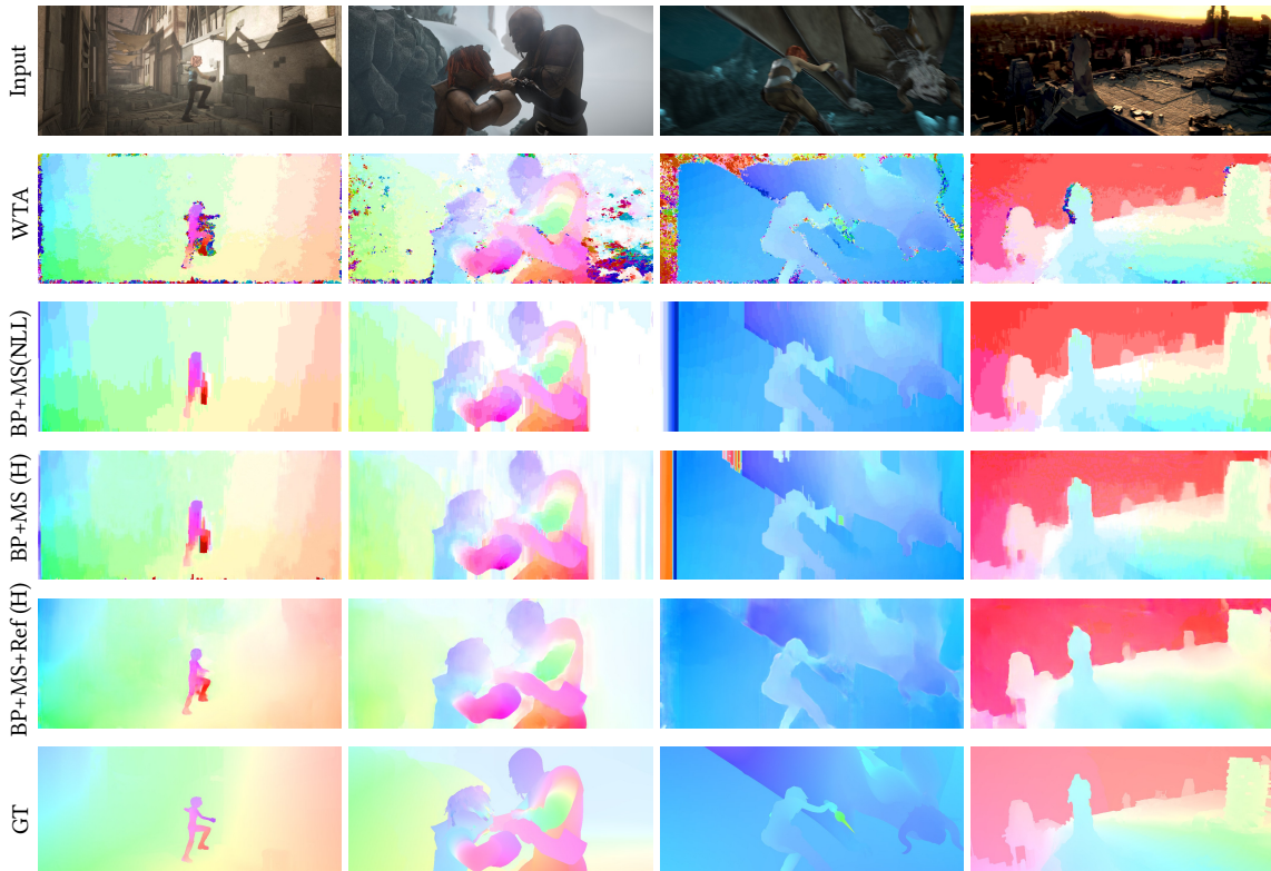
Figure 4.12: Qualitative ablation study for optical flow. The WTA result clearly shows occluded regions (the noisy regions), while our model is able to successfully inpaint these regions. Note that the details increase from top to bottom.
