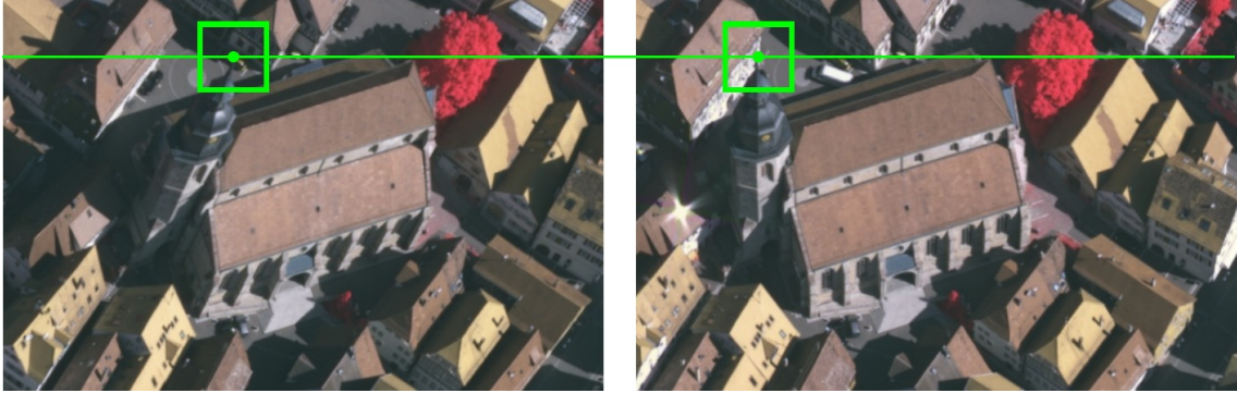
Figure 1.1: Stereo matching on rectified images. The left image shows the reference image together with a reference point/patch. The task is to find the corresponding point in the right image on the epipolar line. The green line depicts the epipolar line, which corresponds to an image row.
