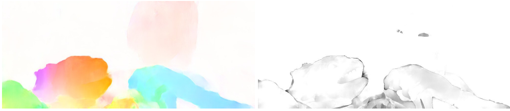
Figure 4.11: Left: Qualitative optical flow results on the Sintel validation set. Right: Visualization of the endpoint error, where white=correct and darker pixels are erroneous.
