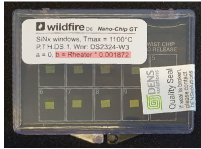
Figure 2.2.: Box of Nano-Chips . The ones we are using are covered with a <20 nm thick \text{SiN}_x membrane. On the label the coefficients a and b for Eq. (2.1) are given.
