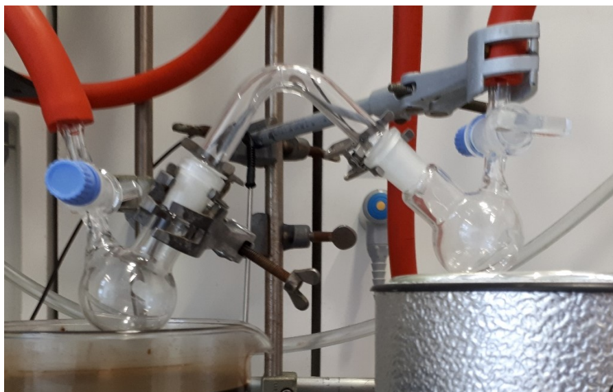
Figure 30 General setup for the condensation-trapping experiments; the left flask contains the rhenium catalyst, the nitrate or nitrite salt and can be heated in the oil-bath; the right flask contains DMS in \text{CD}_3\text{CN} and is cooled down, generally to -100\text{ }^\circ\text{C} or -196\text{ }^\circ\text{C} , in order to trap volatile compounds generated in the left flask
