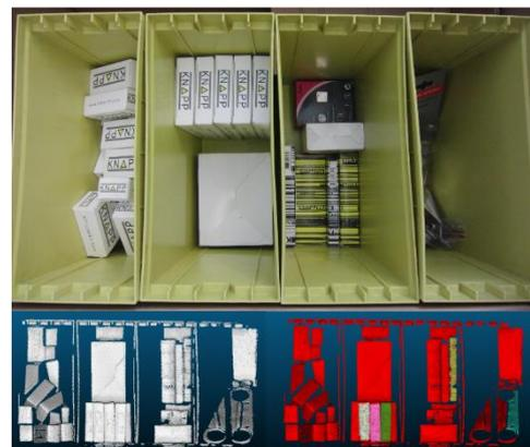
Figure 111: Test container for the measurement by ENSHAPE (top), 3D point cloud (bottom left) and segmentation (bottom right)
