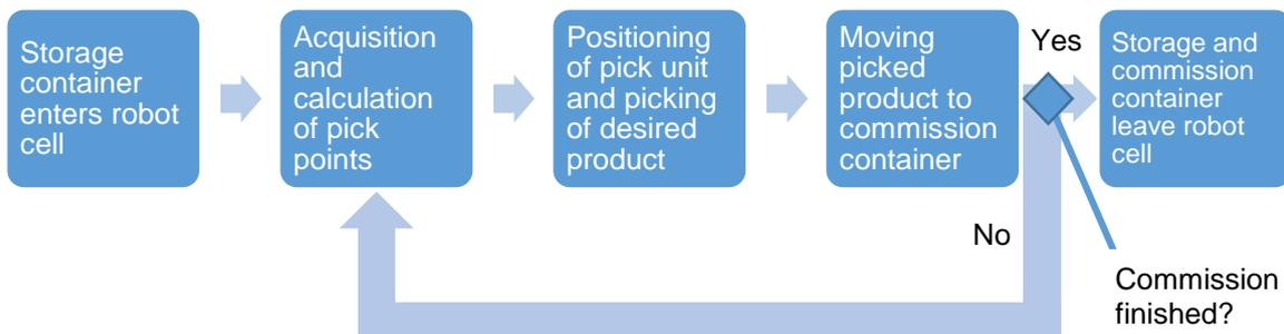
Figure 2: Picking process of Pick-it-easy Robot by KNAPP
