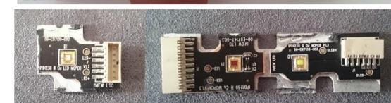
Figure 99: Disassembly process of the Lightcrafter 4500 to change the LEDs
