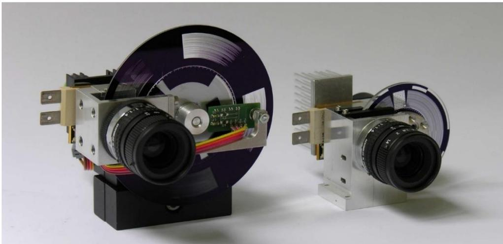
Figure 52: First (left) and second (right) generation of analogue pattern projection unit. (Wissmann, 2013)
