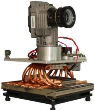
Figure 110: Lightcrafter 6500 (top) (TI, 2014) and STAR-065 (bottom) (VIALUX,
