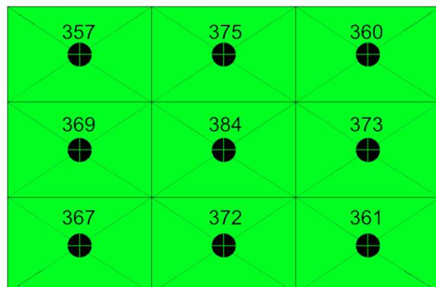
Figure 101: Measurement M3, green high-power LED. Measured values are in Lux.
