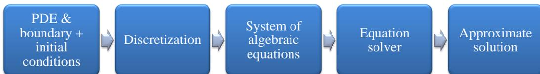
Figure 2.12: Overview of computational solution procedure [53].
