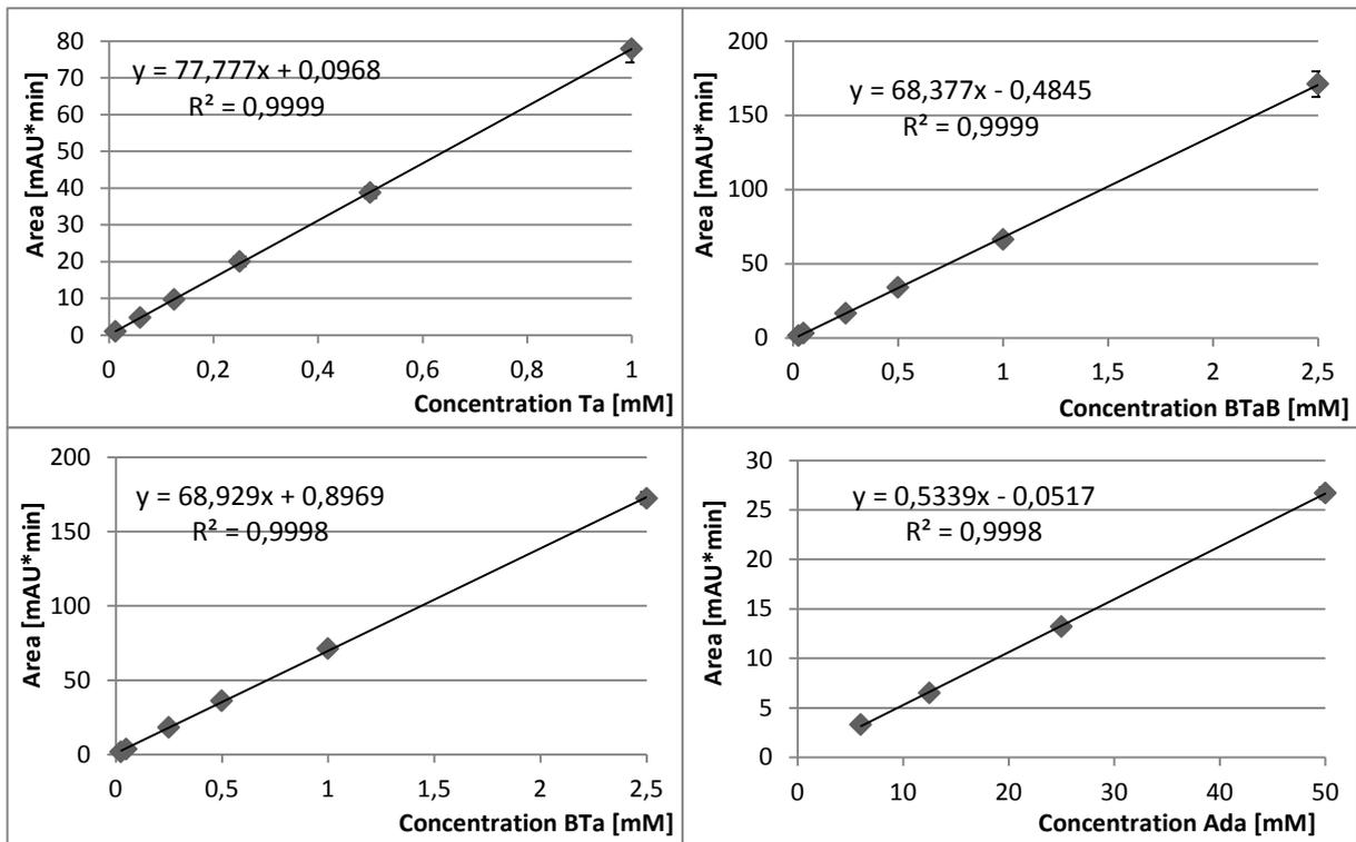
App. Figure 1: Ta, BTaB, BTa and Ada standards for quantification of degradation products created by enzymatic hydrolysis of AAC. The standards were dissolved in potassium phosphate buffer (0.1 M, pH 7.0) and a methanol precipitation was performed.
