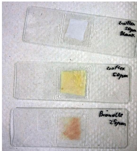
Figure 23: Comparison of ecoflex and Bionolle foil pieces that were incubated for 3 weeks in biogas sludge to a blank. From top to bottom: ecoflex 50  $\mu\text{m}$  blank; ecoflex 50  $\mu\text{m}$ ; Bionolle 25  $\mu\text{m}$ .
