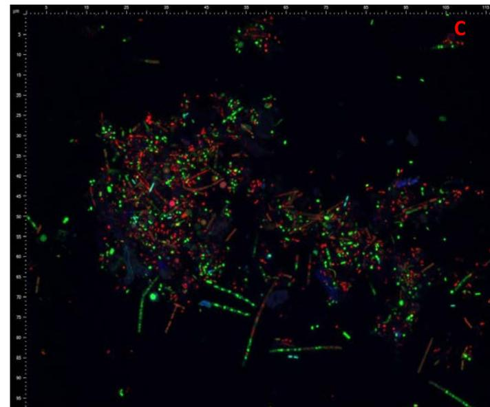
Figure 24: All images at maximum projection of all stacks and channels. **A:** Bionolle 25  $\mu\text{m}$ . **B** and **C:** ecoflex 50  $\mu\text{m}$ . There is a high abundance of living and dead cells which are likely linked together in biofilms. The blue signals are an indication for the presence of cofactor F350 which is mainly present in methanogenic organisms.
