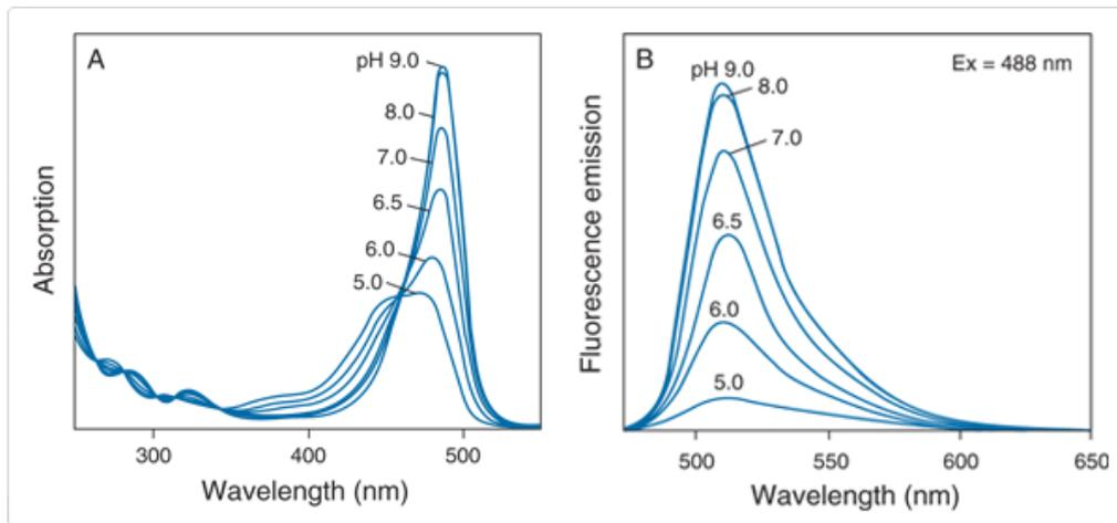
Figure 4: Absorption and fluorescence emission spectra of fluorescein at different pH values [28].
