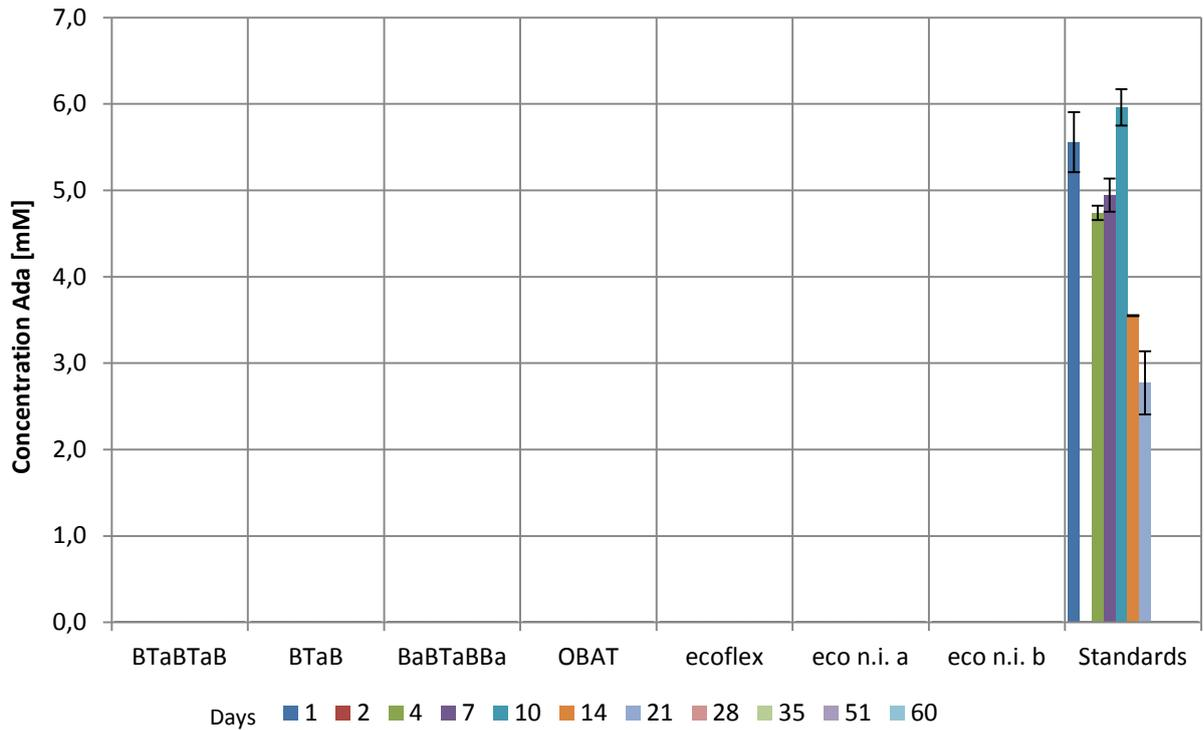
App.Figure 5: Ada concentrations in the sludges measured by HPLC. The Standards batch had an initial Ada concentration of 6.6 mM.
