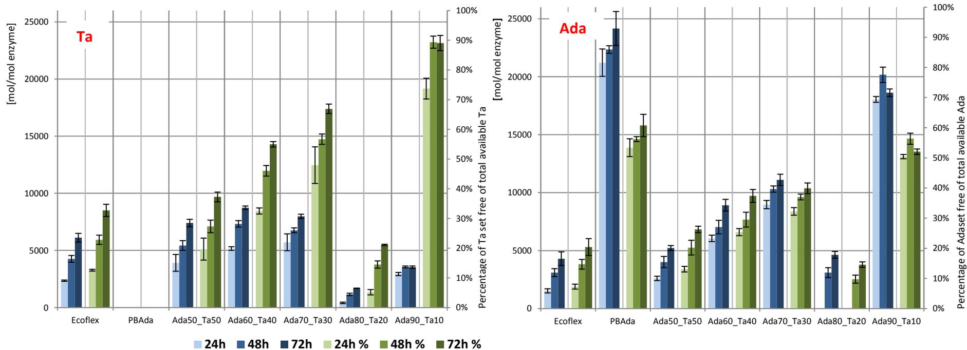
**Figure 11: Hydrolysis products of different model substrates released by ThC\_Cut1. On the primary vertical axis, the mole products that are released per mole enzyme are displayed. On the secondary vertical axis, the percentage that is enzymatically set free of the total available amount is depicted. The degradation was carried out with an enzyme concentration of 0.6  $\mu\text{M}$  at 50° C. The reaction was stopped after 24h, 48h and 72h to show the progression of the degradation.**
