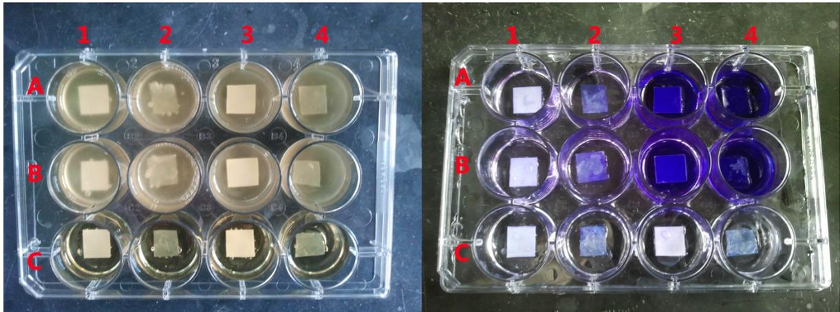
Figure 21: Left side: Incubation of polymer foils with *E. coli* and *S. aureus*. Right side: crystal violet remaining on the samples after washing with H<sub>2</sub>O. Rows A and B are duplicates, C is the control with sterile medium. Column 1: *E. coli* 400  $\mu\text{m}$  ecovio; Column 2: *E. coli* 50  $\mu\text{m}$  ecoflex; Column 3: *S. aureus* 400  $\mu\text{m}$  ecovio; Column 4: *S. aureus* 50  $\mu\text{m}$  ecoflex
