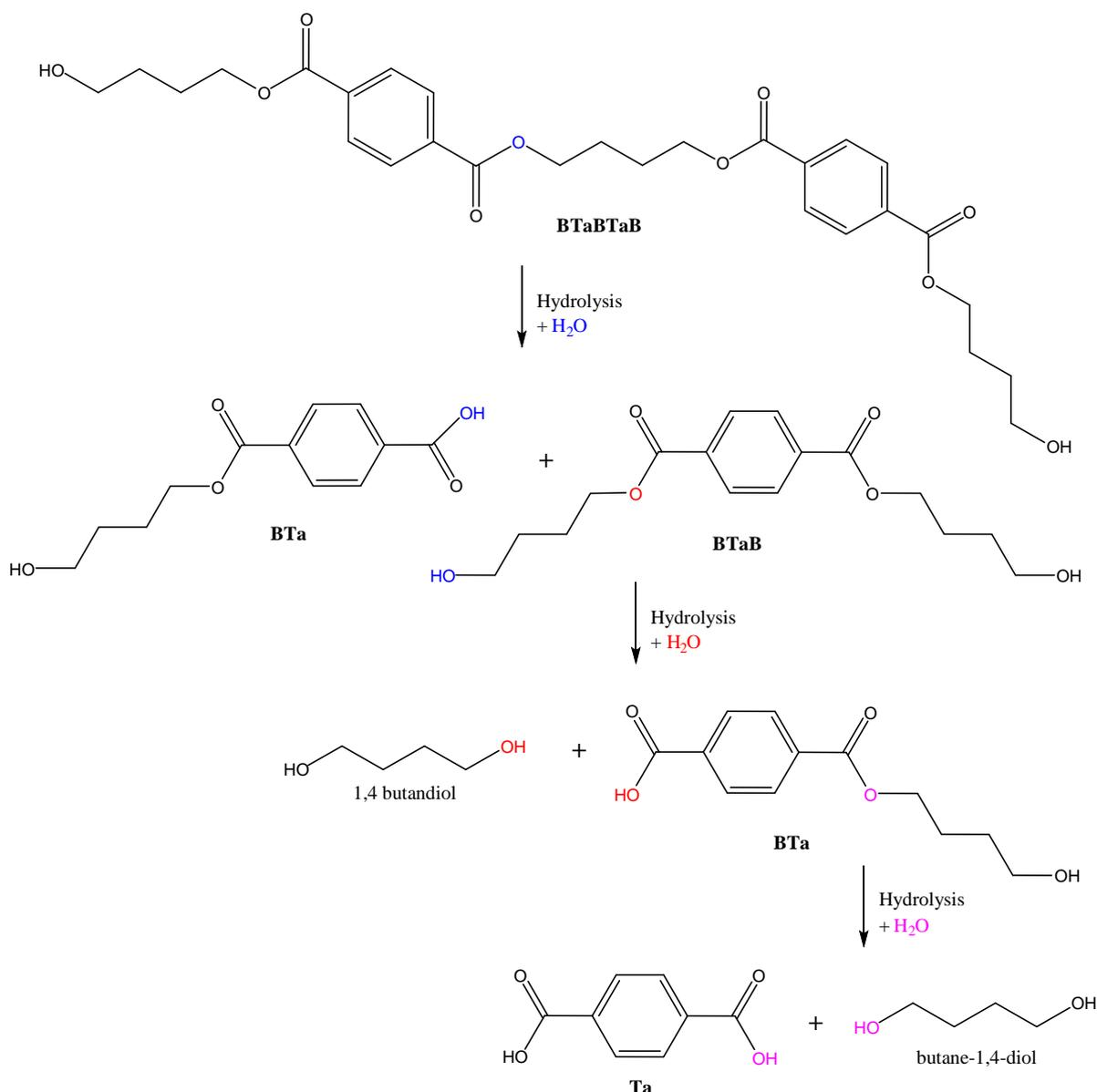
Figure 10: Schematic representation of the hydrolysis of a possible ecoflex degradation intermediate. The ester bonds are enzymatically hydrolysed and smaller products emerge which can be quantified by HPLC.
