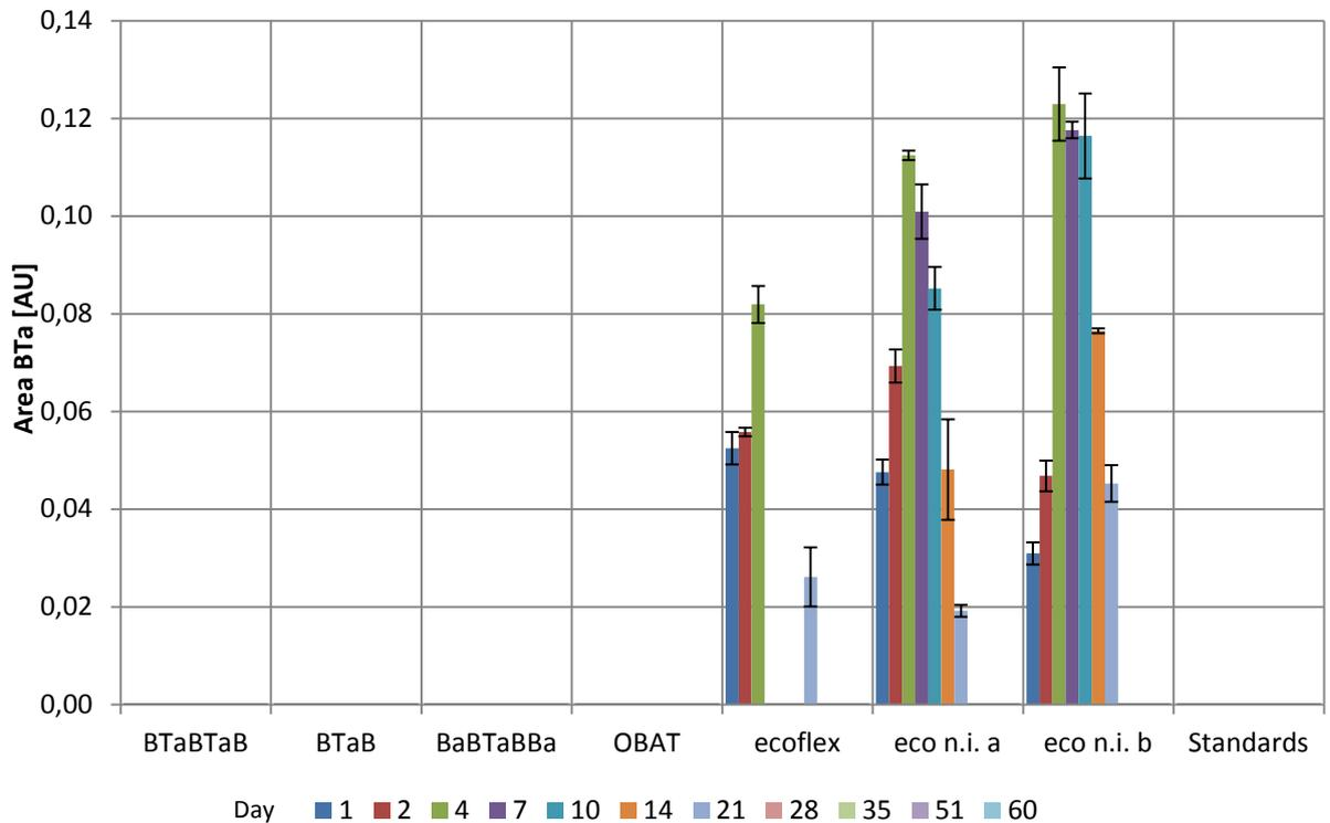
App.Figure 6: BTaB concentrations in the sludges measured by HPLC.
