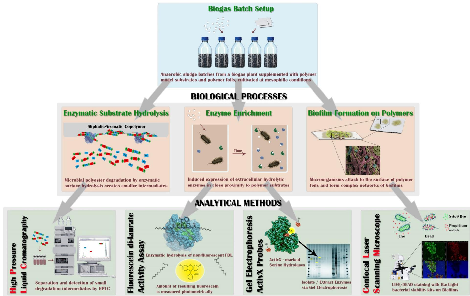
Figure 8: Overview about the setup, biological processes and detection methods involved in the anaerobic biogas sludge batch experiment. Polymer model substrates and polymer foils were used to induce expression of polymer hydrolysing enzymes. The hydrolysis products, enriched enzymes and the biofilm formation were analysed: The hydrolysis products by HPLC, the enzyme enrichment with an activity assay and PAGE, and the biofilm formation was observed with confocal microscopy.
