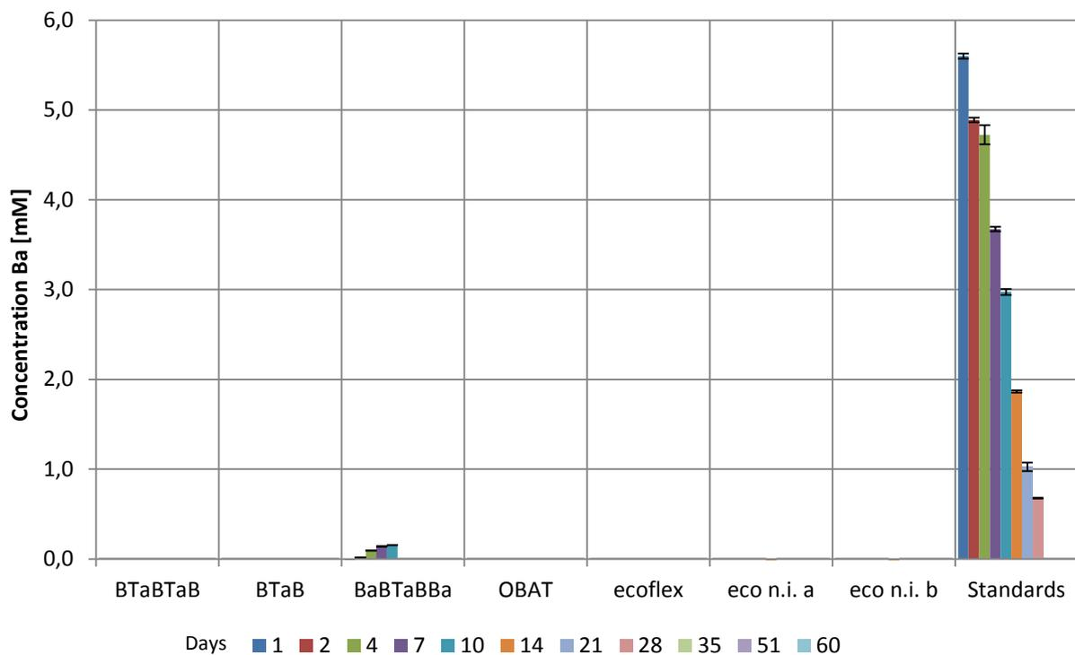
App. Figure 4: Ba concentrations in the sludges measured by HPLC. The Standards batch had an initial Ba concentration of 6.4 mM.
