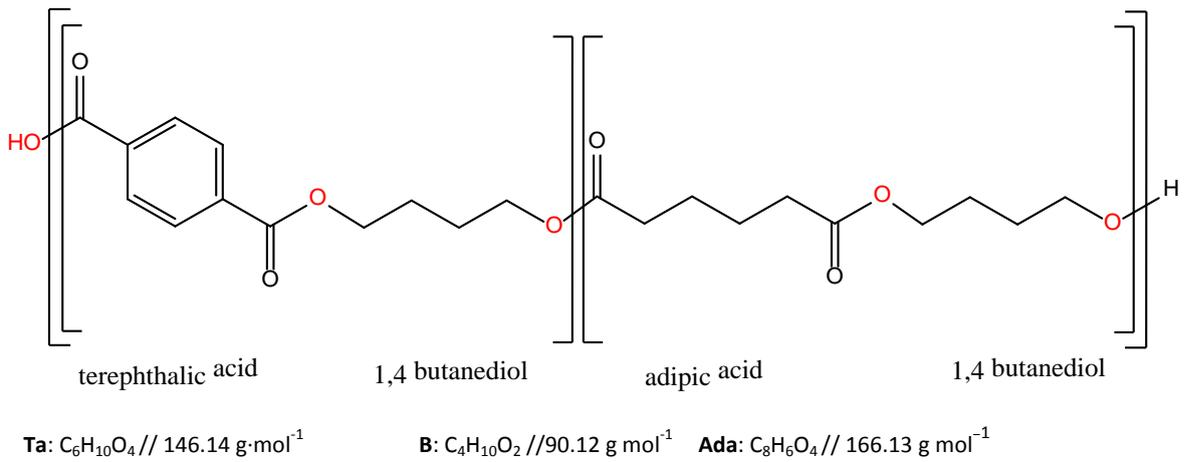
**Figure 2: Structure of the aromatic aliphatic copolyester ecoflex with the ester bonds marked in red and molecular weights of terephthalic acid, 1,4 butanediol and adipic acid.**
