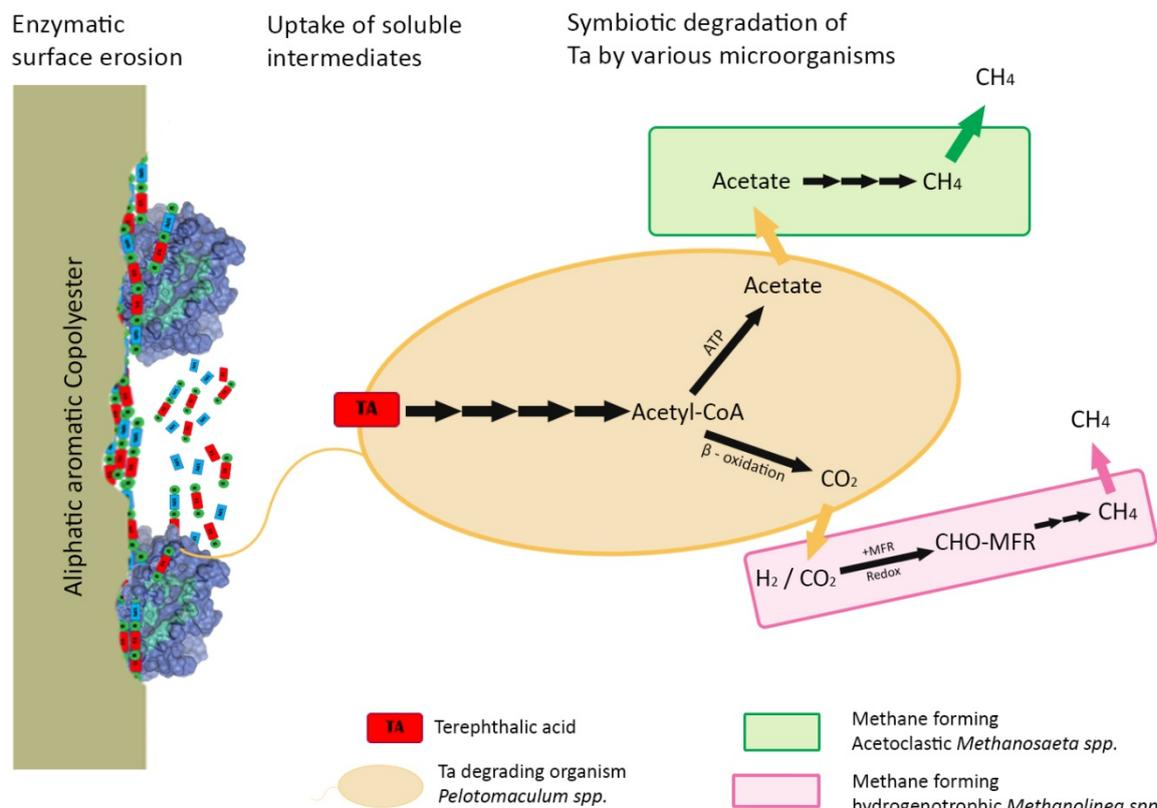
**Figure 19:** Schematic depiction of Ta degradation in a mixed microbial culture. Polymer chains are degraded in an enzymatic surface erosion process and soluble intermediates like Ta are released. Ta is taken up by Ta degrading organisms like *Pelotomaculum* spp. and through acetyl-CoA in different pathways acetate and CO<sub>2</sub> are formed, which are secreted and used by other organisms to form methane. [diagram modified after [59], [60]]
