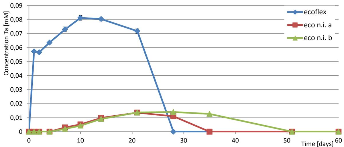
**Figure 18: Comparing the metabolic lag phases of different sludges containing ecoflex. All three sludges used ecoflex as carbon source; however, their original inoculation sludges had different sources: “ecoflex” was previously used in experiments with other polymeric substrates and was fed with PHA; “eco n.i.a” and “eco n.i.b” were only in contact with maize silage prior to this experiment.**
