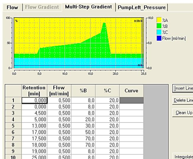
Figure 6: HPLC Gradient was used for the analysis of ecoflex hydrolysis products. A: ddH<sub>2</sub>O, B: acetonitrile and C: 0.1 % formic acid.
