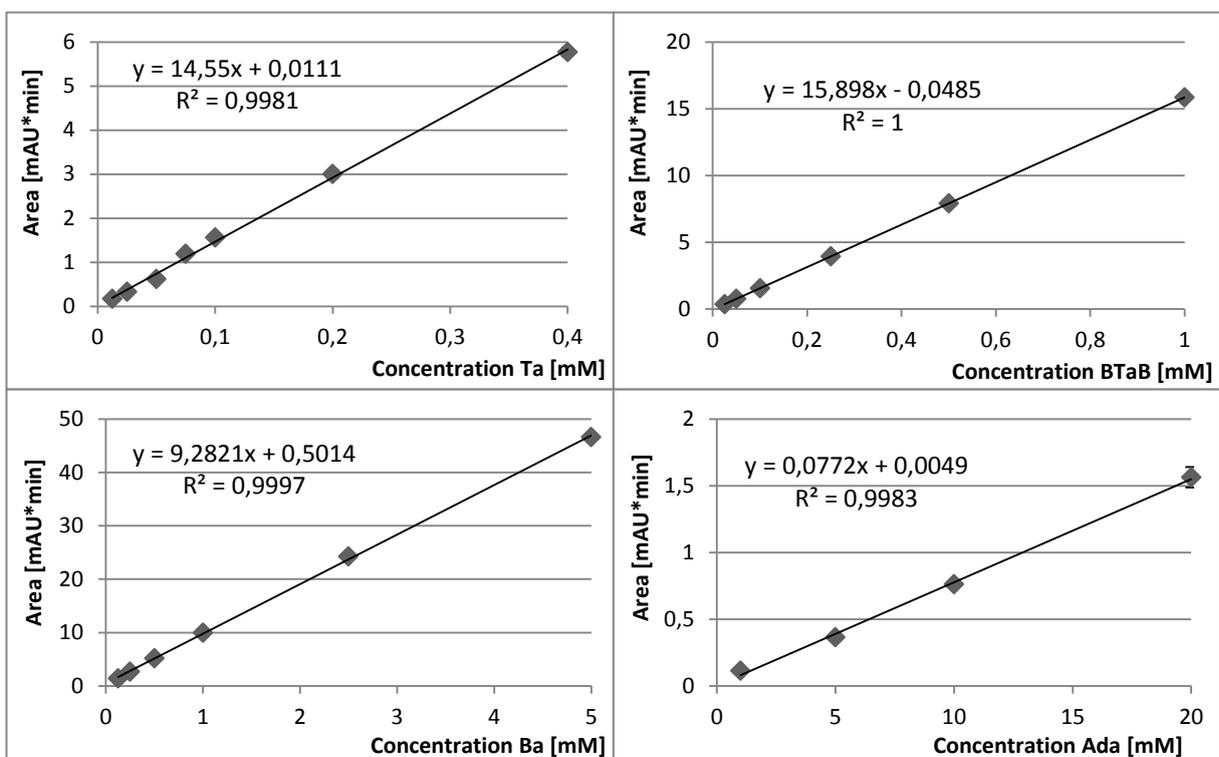
App. Figure 2: Ta, BTaB, Ba and Ada standards for quantification of degradation intermediates in the sludge experiment. The standards were dissolved in potassium phosphate buffer (0.1 M, pH 7.0) and a Carrez clarification was performed.
