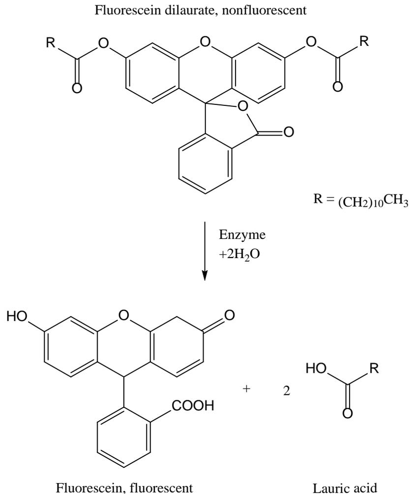
**Figure 3: Enzymatic cleavage of the non-fluorescent fluorescein dilaurate to the fluorescent fluorescein.**
