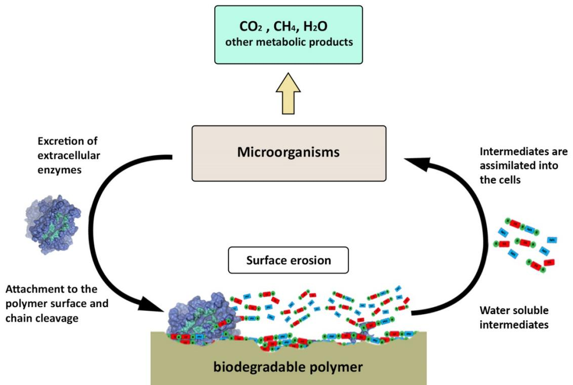
Figure 1: The process of biodegradation of biodegradable polymers. Microorganisms secrete extracellular enzymes which attach to the polymer surface and release water soluble intermediates. These degradation intermediates are then assimilated into the cells where they are metabolized to  $\text{CO}_2$ ,  $\text{CH}_4$  and  $\text{H}_2\text{O}$ . [modified from R.-J. Mueller [3]]
