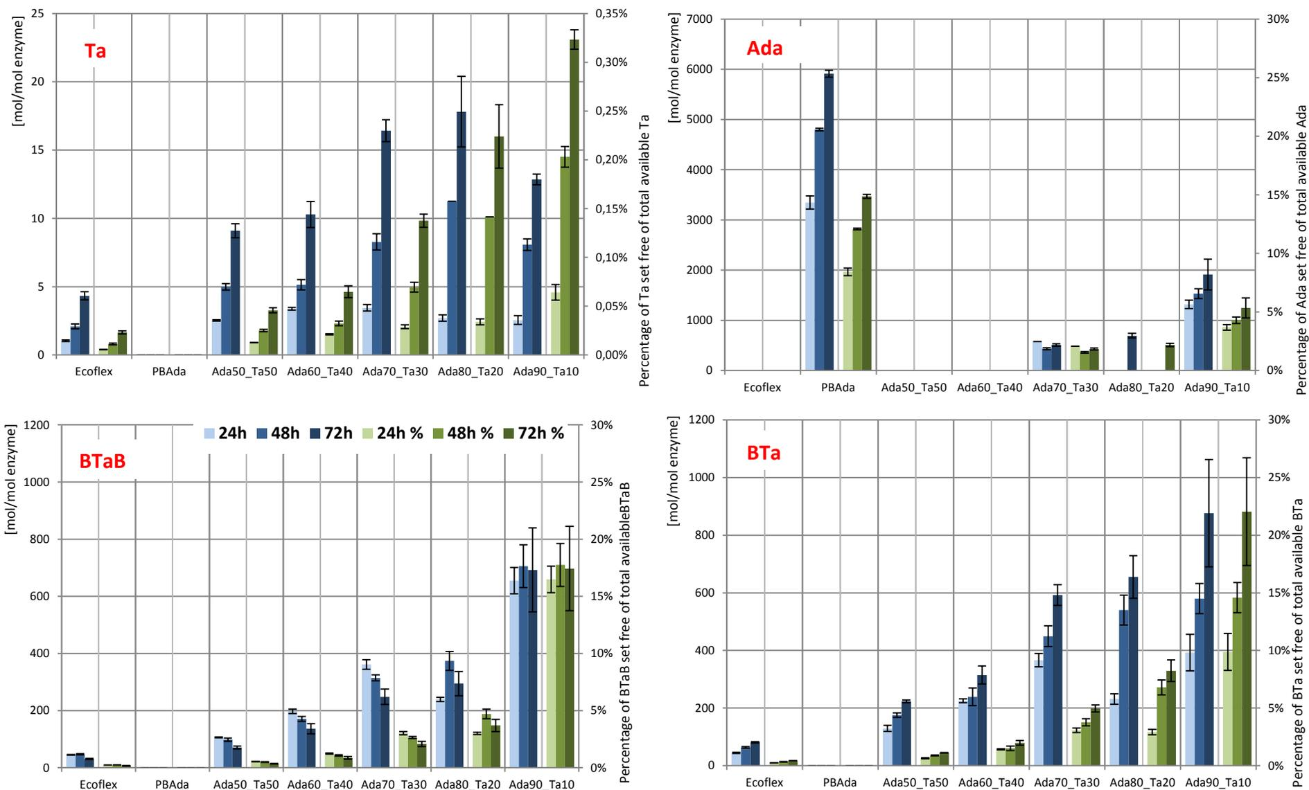
**Figure 12: Hydrolysis products of different model substrates released by CB\_EstA. On the primary vertical axis, the mol product that are released per mol enzyme are displayed. On the secondary vertical axis, the percentage that is enzymatically set free of the total available amount is shown. The degradation was carried out with an enzyme concentration of 0.6 μM at 50 °C. The reaction was stopped after 24h, 48h and 72h to show the progression of the degradation.**
