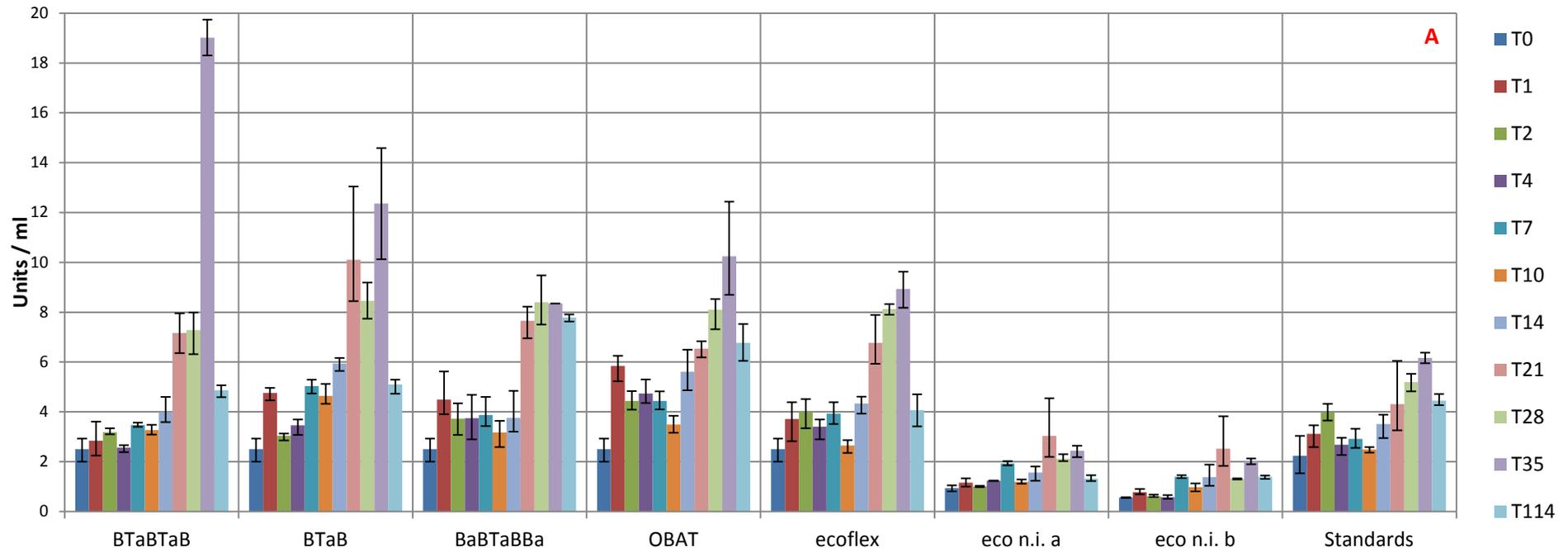
Figure 16: Summary of the esterase activity on FDL in the different sludges obtained from anaerobic batches. "T" is the time passed in days. Diagrams A and B represent the same data, with a correctly proportioned timeline in diagram B. Most of the change in activity was expected in the first week, therefore more measurements were performed in the first 10 days. Afterwards the activity was monitored weekly until day 35. After 114 days the experiment was stopped (not shown in B).
