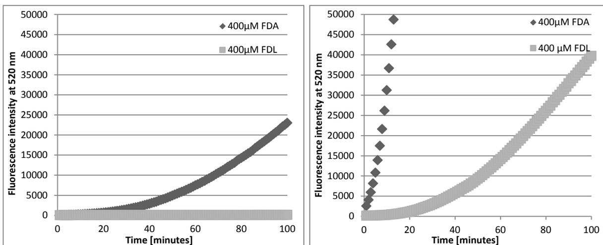
Figure 15: Left side: Autocatalysis of 400 μM FDL or FDA in NaPO<sub>3</sub> buffer pH 7.0. Right side: Enzymatic hydrolysis of 400 μM FDA or FDL in sludge.
