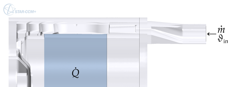
Figure 2.4: Spatially uniform heat injection (heat flux density) at coloured surface.
