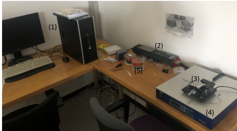
Figure 2.9: Setup for the AFM measurement with the (1) computer, the (2) electronic control unit, the (3) AFM stage, the (4) vibration absorber and the (5) measuring head.
