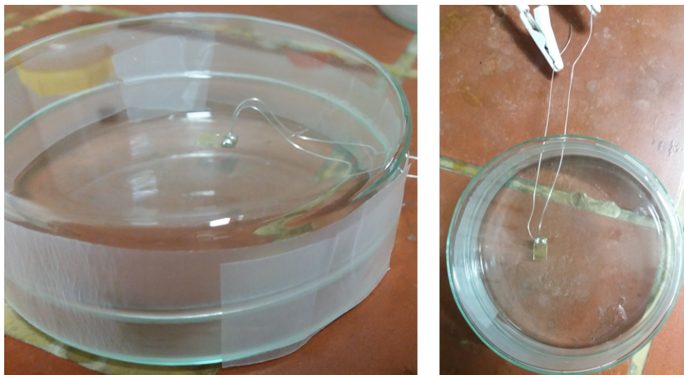
Figure 2.7: Solvent vapor annealing setup from the side (left) and from the top (right). The chamber consists of two Petri dishes connected with a para tape. The wires are connected to a voltage source as can be seen in the right picture.
