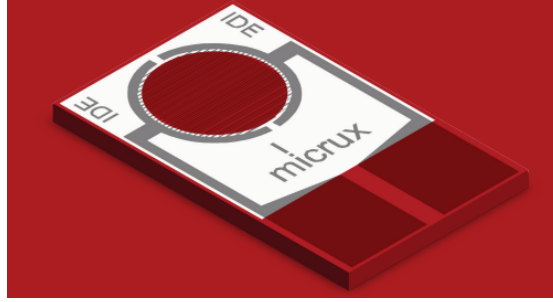
Figure 2.16: Picture of the glass substrate with gold electrodes on it, where the white layer is the SU-8 protective layer.[Inta]
