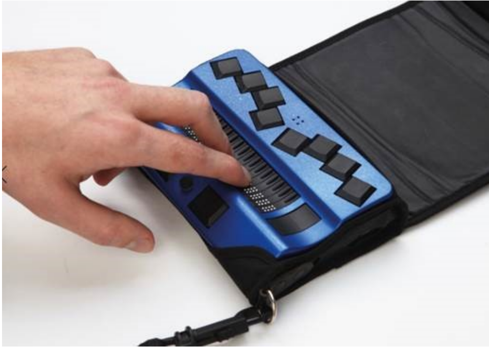
Figure 2.2: Actilino by Help Tech [2021] is a portable Braille display with 16 cells, deployed in a protective carrier bag. [Image provided by and used with kind permission of Help Tech [2021].]
