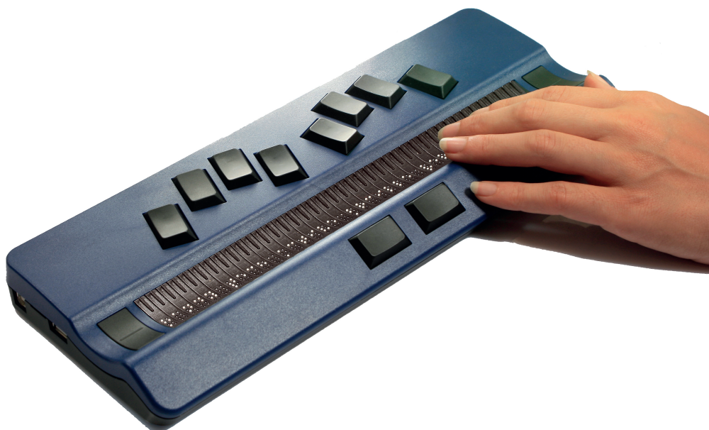
Figure 2.1: Active Braille by Help Tech [2021] is a portable Braille display with 40 cells. The surface of each module is concave to accommodate the shape of a reading finger. Each module incorporates an additional slim key (the Cursor-Routing key) above its Braille cell. Concave navigation keys are located to the left and right of the Braille line. Other keys are located above and below the cells. The device has been turned on, and some of its Braille dots are set. A left hand can be seen towards the right end of the line, reading the displayed Braille content. [Image provided by and used with kind permission of Help Tech [2021].]
