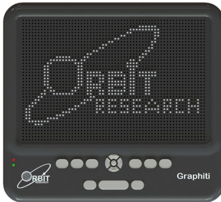
Figure 3.1: Graphiti by Orbit [2021], a portable tactile graphics display with 40×60 pins, viewed from above. Navigation keys are located in front of the pin array. The device is displaying the logo of the manufacturer. [Image provided by and used with kind permission of Orbit [2021].]
