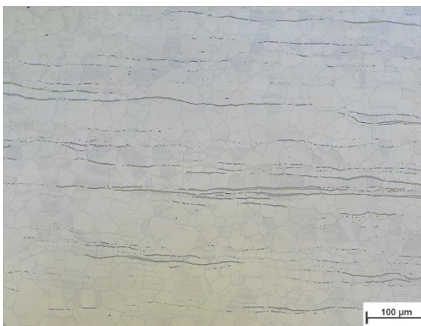
Figure 51. The specimen (Transverse Plane) heat-treated at 1000°C.
