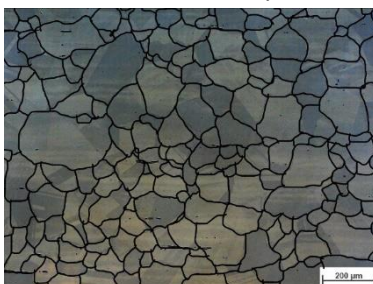
25 (f). LOM image of recrystallized 50% cold-rolled heat-treated at 1200°C – 60 min, the average grain size was measured 81μm.
