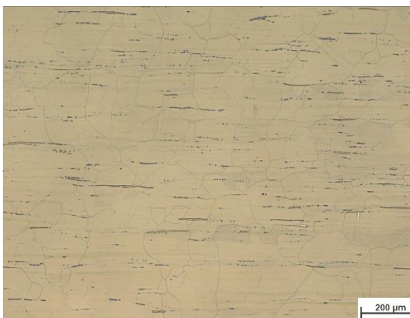
Figure 54. The specimen (Transverse Plane) heat-treated at 1100°C.
