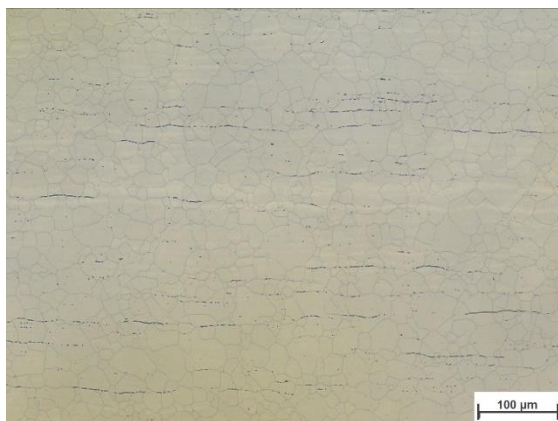
Figure 50. The specimen (Transverse Plane) heat-treated at 900°C.
