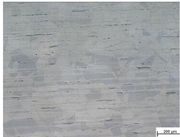
Figure 52. The specimen (Transverse Plane) heat-treated at 1100°C.
