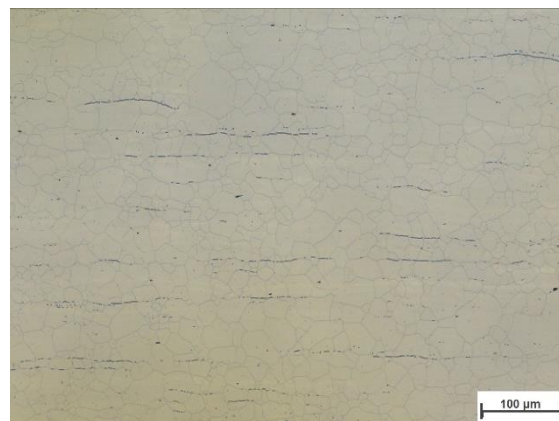
Figure 50. The specimen (Transverse Plane) heat-treated at 900°C.
