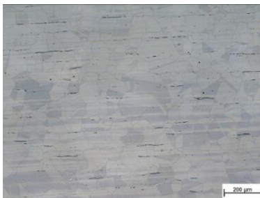
25 (d). LOM image of recrystallized 50% cold-rolled heat-treated at 1100°C – 60 min, the average grain size was measured 59μm.
