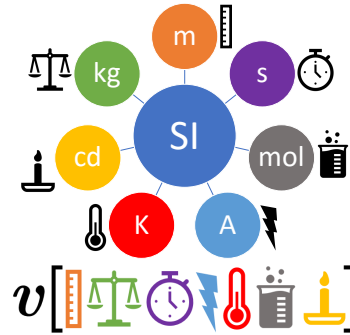
Fig. 1: SI BASE UNITS: m, kg, s, A, K, mol, and cd are the base units in the SI system [ISO 2009; BIPM 2006].
