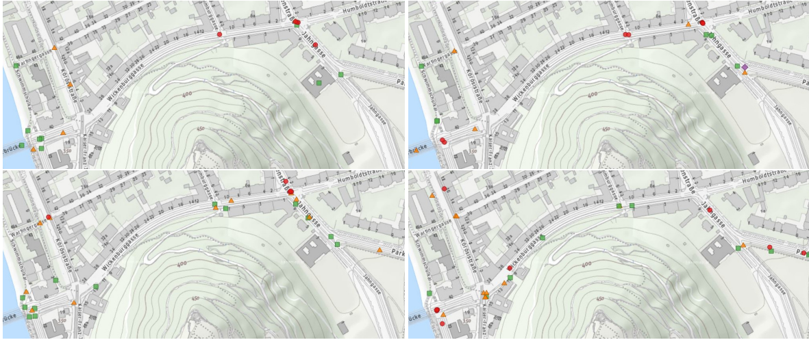
Figure 5.6.: Historical accident data for the years 2013 to 2016, shown for the Wickenburggasse and connecting roads. The red circles represent accidents between passenger cars, the purple diamonds accidents involving powered two-wheelers, the green squares accidents with cyclists and the orange triangles represent accidents with other mixes of participant types. Data taken from Statistik Austria, 2020 and basemap.at
