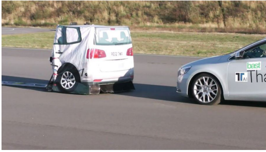
(a) Testing of rear-end collision mitigation systems, Seiniger and A. Weitzel, 2015. (b) An overrunable test platform allowing free control of pedestrian motion, Seiniger and A. Weitzel, 2015.
