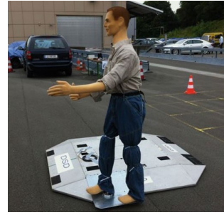
(a) Testing of rear-end collision mitigation systems, Seiniger and A. Weitzel, 2015. (b) An overrunable test platform allowing free control of pedestrian motion, Seiniger and A. Weitzel, 2015.
