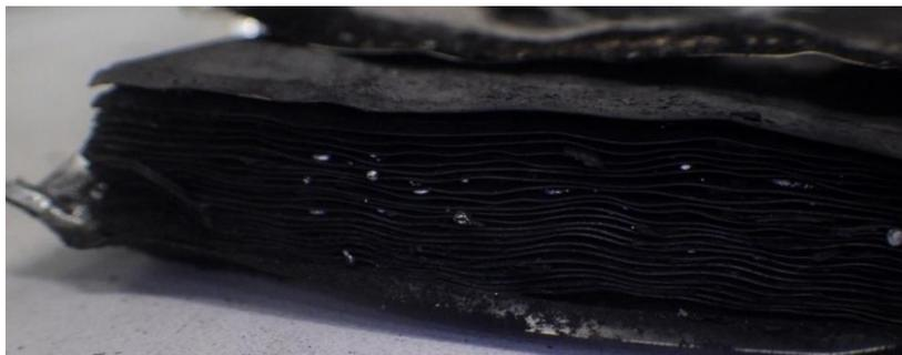
**Figure 26: The pouch cell after TR was opened on the welded sides. Droplets were visible between the stacked cell layers [5].**
