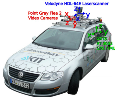
Fig. 1. Recording platform of the KITTI dataset. A standard passenger car is equipped with multiple cameras, a LIDAR scanner and a GPS localization system. Picture obtained from [9].
