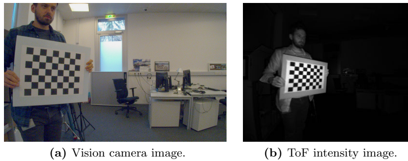
Figure 4.11: ToF and vision camera images, utilized to estimate their relative alignment.
