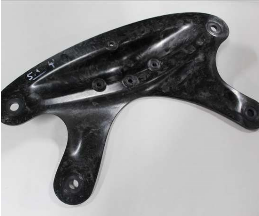
Figure 4 Transmission cross member of a car out of a SMC material [9]
