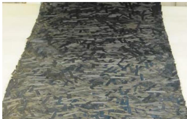
Figure 3 Semi-finished CF-SMC material before the SMC-Process
