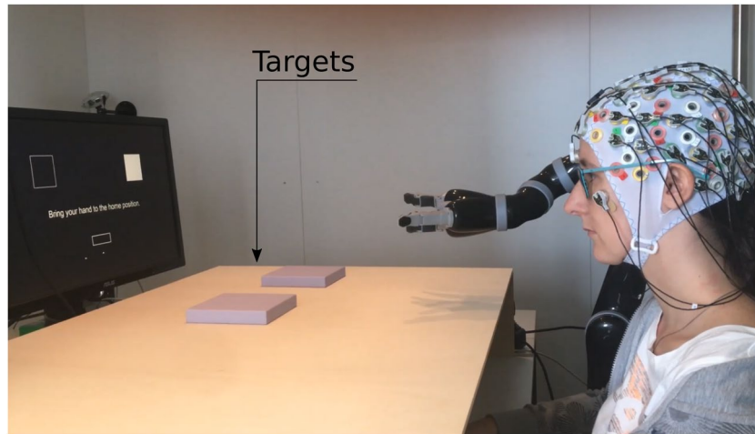
Figure 1. Experimental setup. In this figure, the robot is at its home position. The squares on the screen represent the physical targets (violet cuboids) on the wooden structure. The rectangle on the bottom part of the screen represents the participant's hand home position and the text above it states 'Bring your hand to the home position.' Inside the wooden structure, there is a Leap Motion device (not visible here) used to track the participants' right hand movement.
