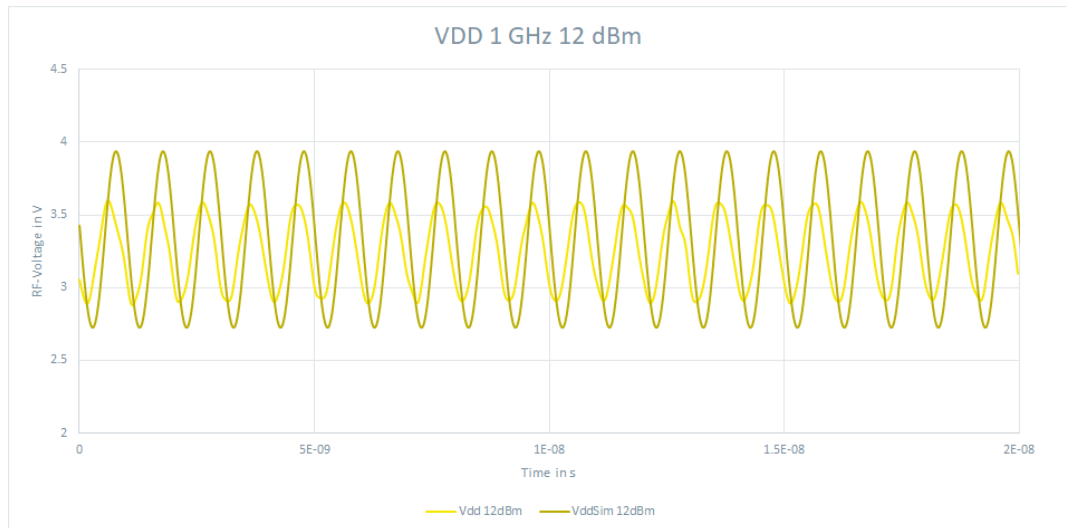
Figure 4.25: DPI measurement of interference signal vs simulation, 12 dBm, 1 GHz
