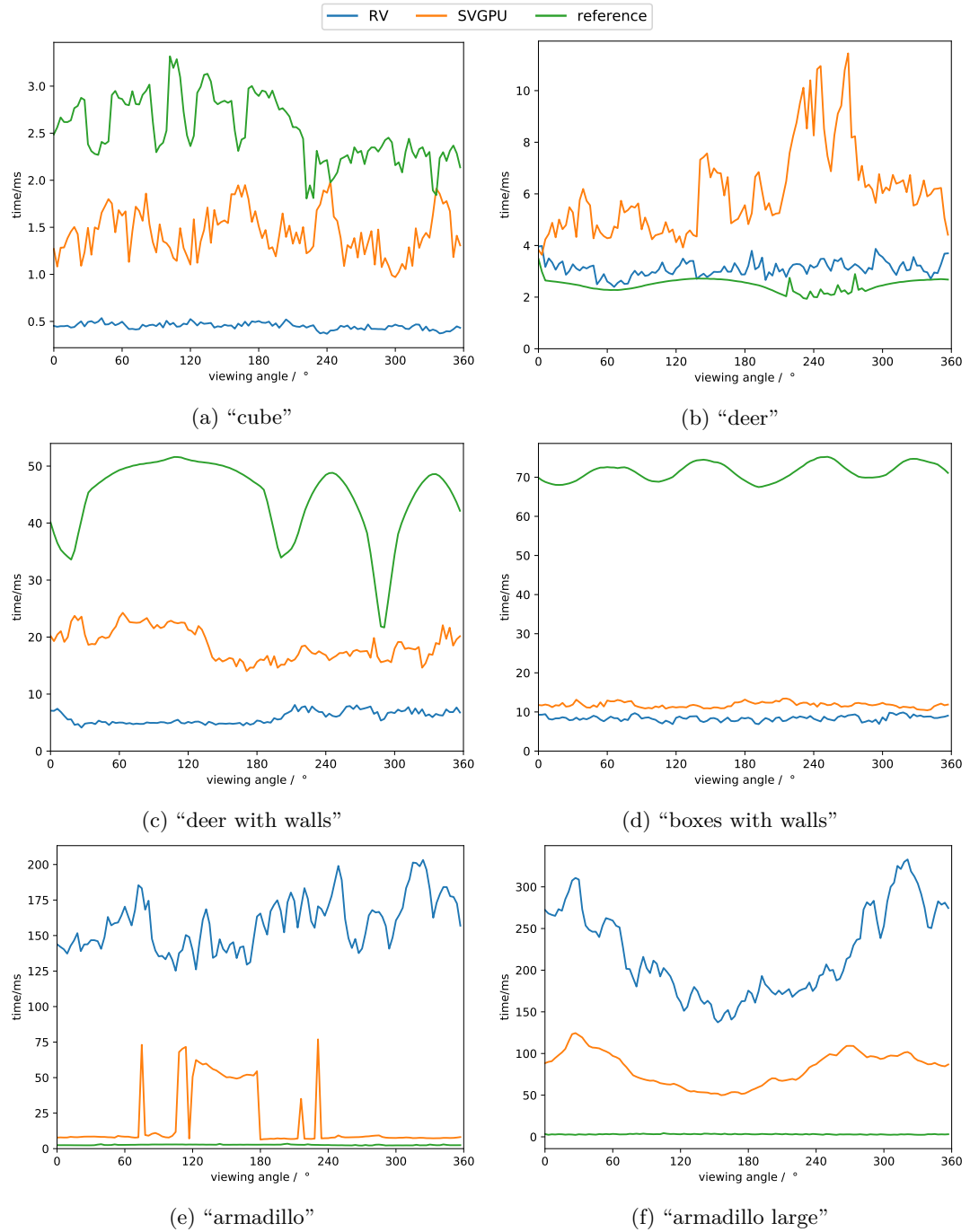
Figure 7.20.: Average runtime of RV, SVGPU and the OpenGL reference method when processing increasingly large scenes. While analytic methods outperform the OpenGL reference on simple scenes, the situation is reversed for very complex scenes. Note, however, that analytic methods can potentially be extended to cover a range of multiple viewpoints which is not possible with the rasterization-based reference. While RV is faster than SVGPU for scenes of moderate complexity, it seems that SVGPU would outperform RV in very large scenes such as “armadillo”. However, if we recall the results from chapter 7.2.1, we note that SVGPU failed to produce correct results in these large scenes which explains the suddenly faster runtime.
