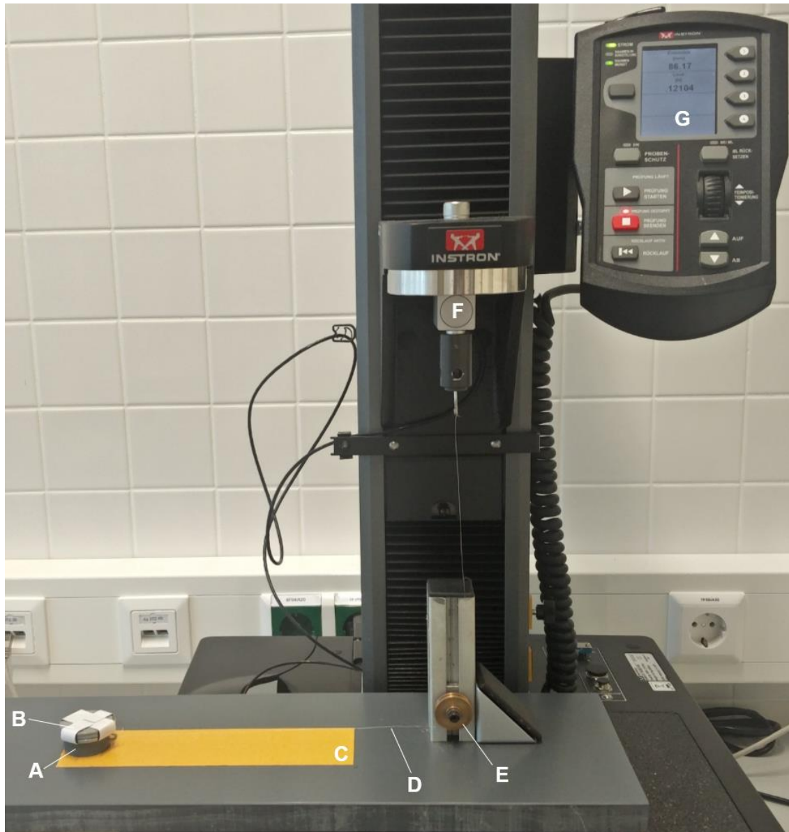
Figure 1. Schematic illustration of the in vitro gliding system developed in this work: (A) testing disc, (B) weight, (C) gliding region, (D) nylon cord connecting the disc to the load cell, (E) height-adjustable wheel with position stopper, (F) load cell, (G) software display.
