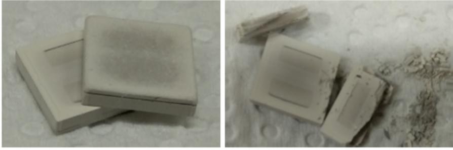
Figure 37: Components WITH inner electrodes after the measurement with modified temperature- and atmosphere settings.
