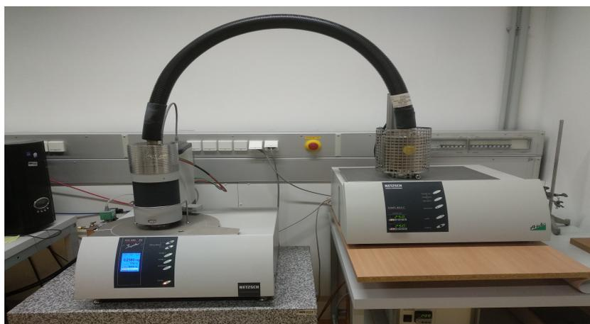
Figure 10: Final experimental setup with the STA on the right side and the MS on the left side.
