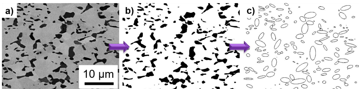
Figure 18: Procedure to obtain the shape factors in \alpha -phase for the Ti-17.
