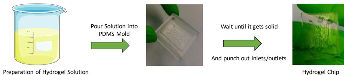
**Figure 3.4:** General steps of hydrogel solution preparation. Firstly, the hydrogel solution mixture was prepared and poured into PDMS molds. After solidifying step, inlets/outlets were punched out from the hydrogels.
