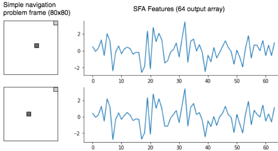
Figure 25: Linear Regression on SFA features performed on simple navigation game. Agent's x and y coordinates, as well as goal position are coded in SFA features represented as 64 output array
