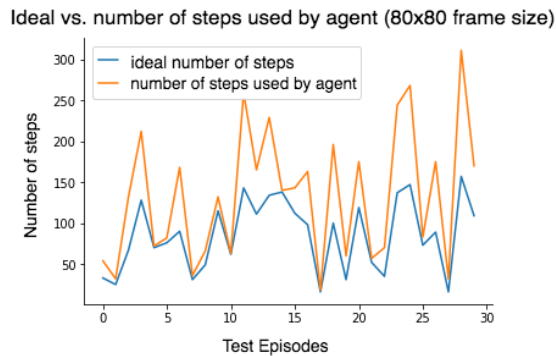
Figure 21: Ideals vs. number of steps used by agent over episodes. According to start agent position the smallest distance is calculated (calculated by Manhattan distance) between the agent and a goal. Then this distance is compared with the number of steps which are done per current epoch.
