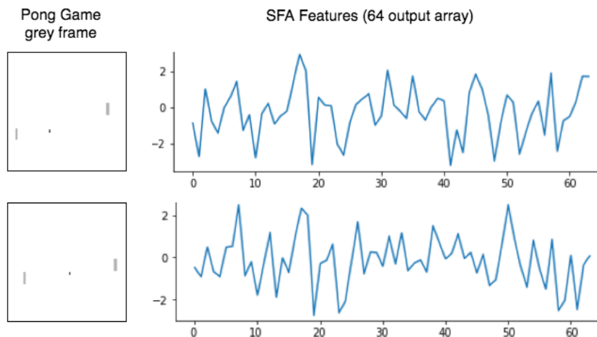
Figure 34: Two SFA feature vectors together with their Pong images are represented as a grey-scale, where 64 elements are used as a size of SFA demonstration. This way, every game frame is re-scaled from the size 80 \times 80 to 64 \times 1 .
